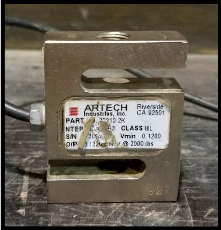
**FIGURE 2.33: ARTECH 20210-2K LOAD CELL**
