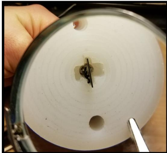
**FIGURE 2.15: BENDER ELEMENT NESTED IN HOUSING (MOAT NOT CUT YET)**
