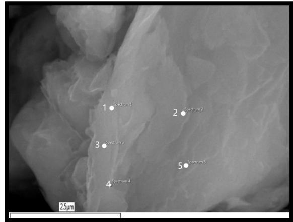
**FIGURE 3.30: SEM IMAGE OF MUSCOVITE SHEETS (CONTROL, A3, 20K MAGNIFICATION)**
