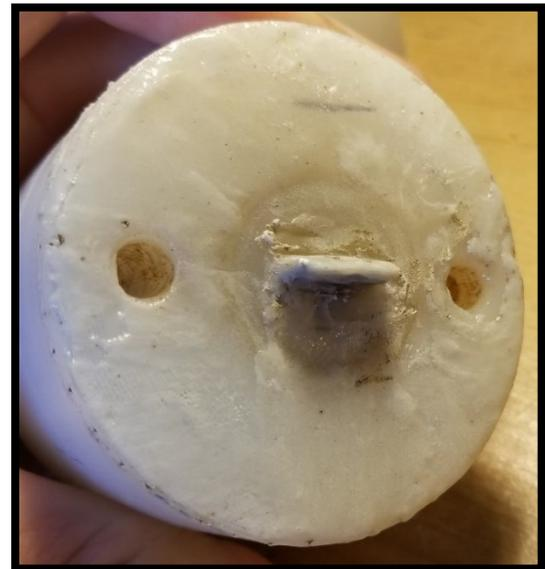
**FIGURE 2.16: COMPLETELY ASSEMBLED BENDER ELEMENT WITH EPOXY COATING**
