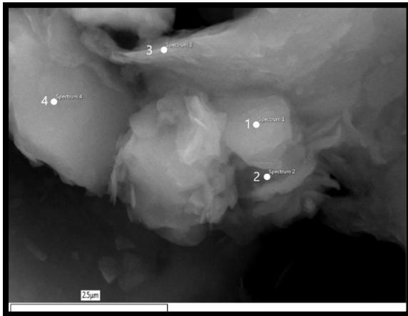
**FIGURE 3.35: SEM IMAGE OF MUSCOVITE SHEETS (BARREL 2, A2, 20K MAGNIFICATION)**
