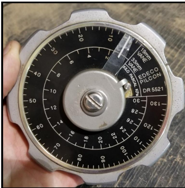
**FIGURE 2.37: EDECO PILCON SHEAR VANE HAND TESTER**
