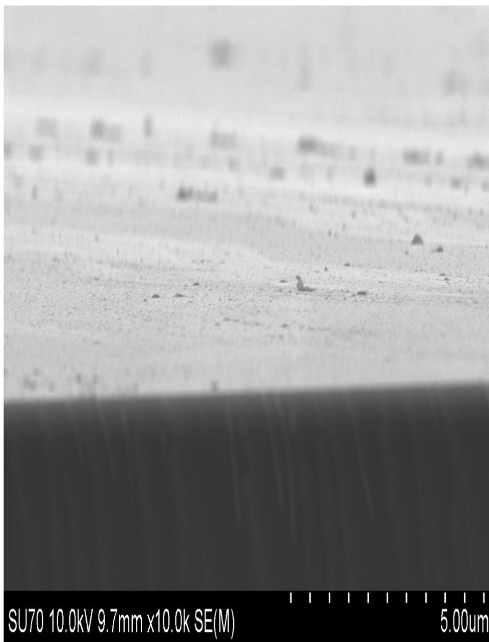
**Figure 34: SEM Surface-View of GaN Growth at 225mTorr, 800W**
