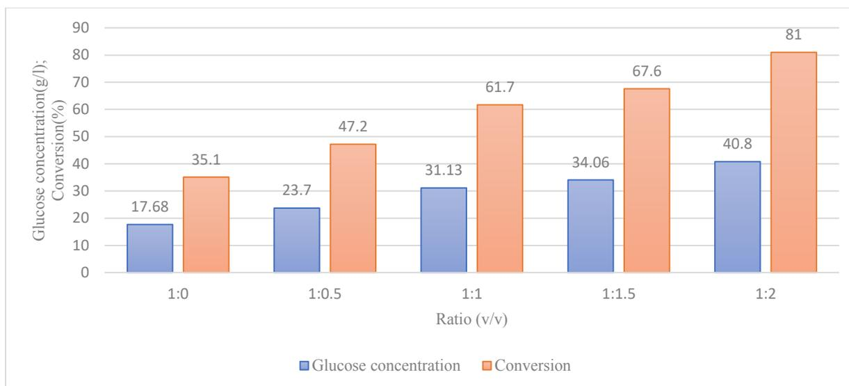
**Figure 4.9: The concentration of glucose and conversion factor as a function of cellulase to  $\beta$ -glucosidase enzyme ratio at 4.5 pH, 40°C temperature, 10% solid loading and 20FPU/g substrate cellulase loading.**
