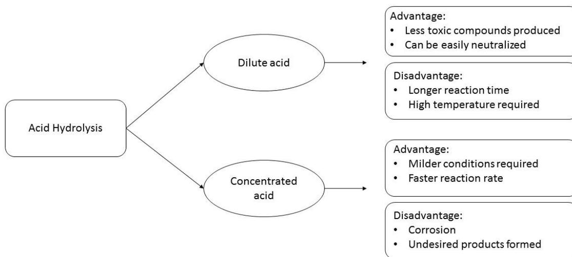
**Figure 2.6: Advantages and disadvantages of acid hydrolysis**
