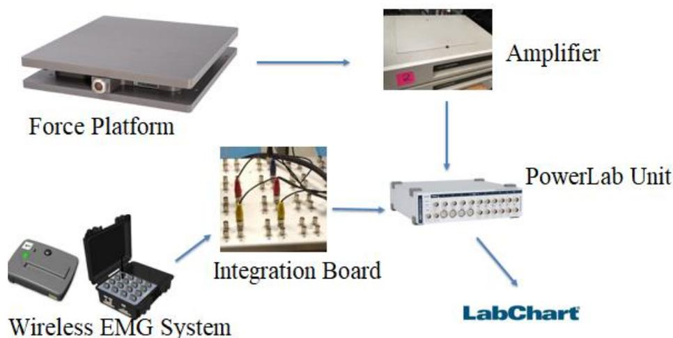
*Figure 6.* Instrumentation set-up. This figure visually represents the configuration of all instruments. The force platform was connected to the amplifier, of which three channels were fed to the PowerLab Unit. The wireless EMG system was connected to the PowerLab unit via an integration board, with five channels being fed into the unit. LabChart® data collected data from both the force platform and wireless EMG system in real time.
