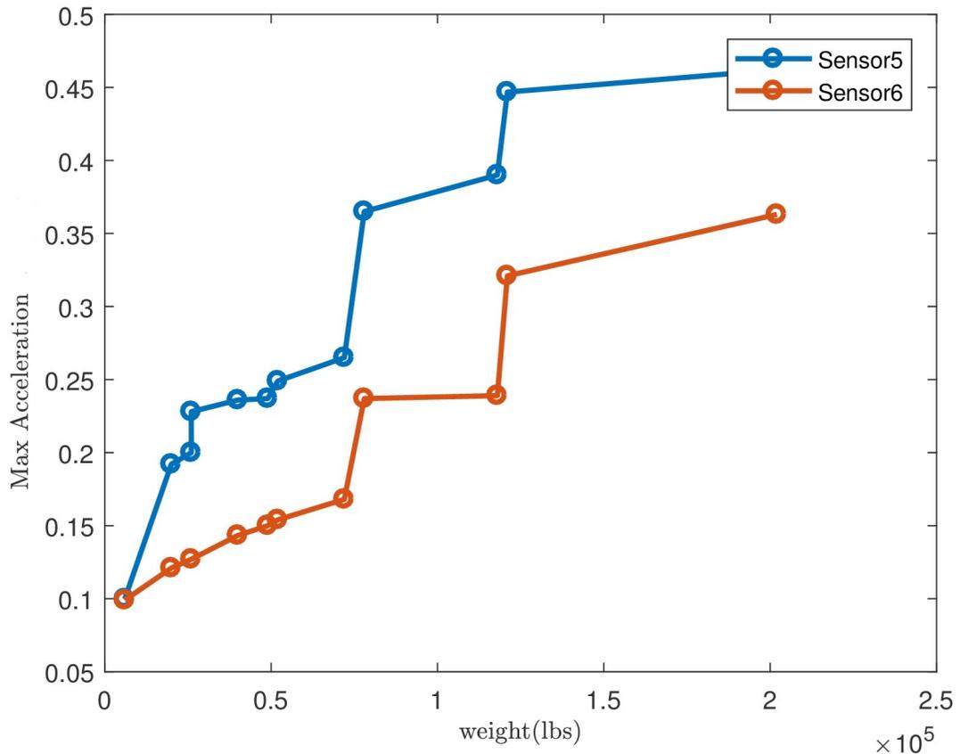
Figure 3.6: Peak vibration response of mid-span sensors under different traffic.
