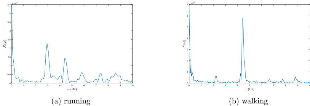
Figure 4.5: Fourier spectra of measured data during running and walking.
