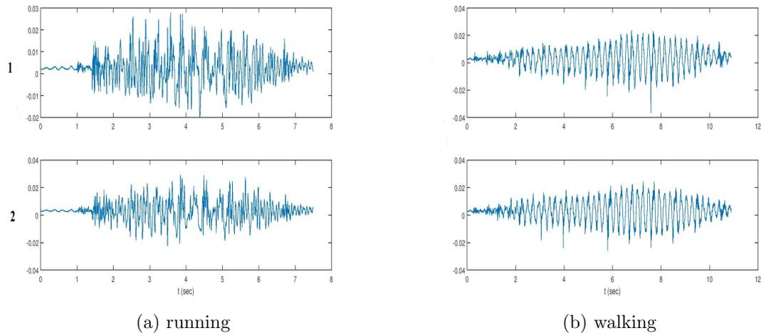
Figure 4.4: Typical vibration data of sensor 1 and sensor 2 during running and walking.
