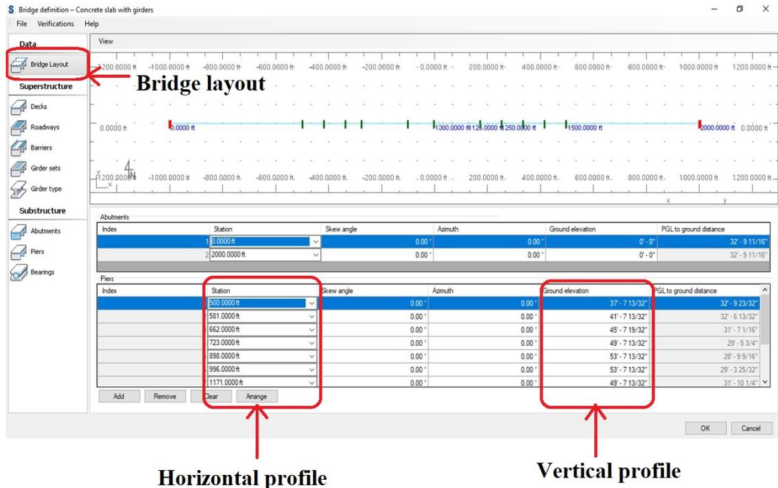
Figure 3.10: Layout of the bridge in Revit®.
