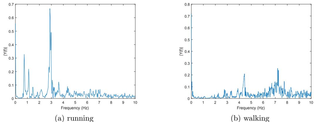
Figure 4.13: Modal responses of foot bridge during running and walking.
