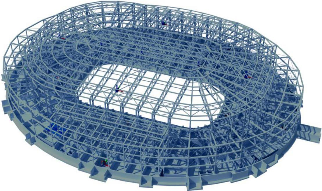
Figure 1.5: BIM model of the Maly Ice Arena in Sochi [47].
