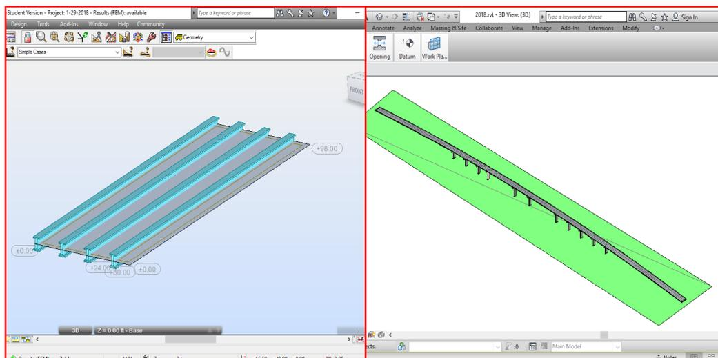
Figure 2.3: Robot structural analysis<sup>®</sup> and the Revit<sup>®</sup> model.
