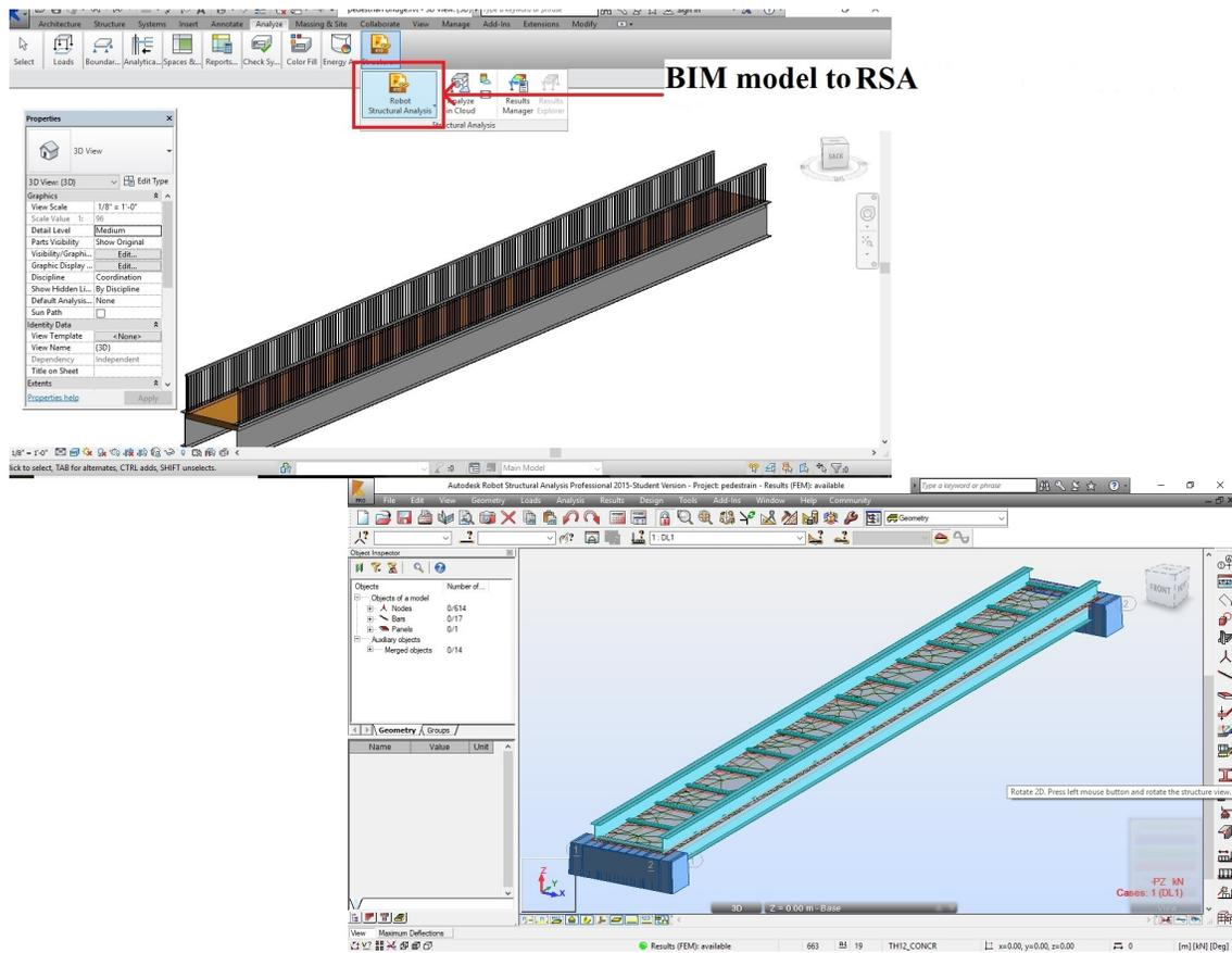
Figure 4.9: Integrated analysis in RSA®.
