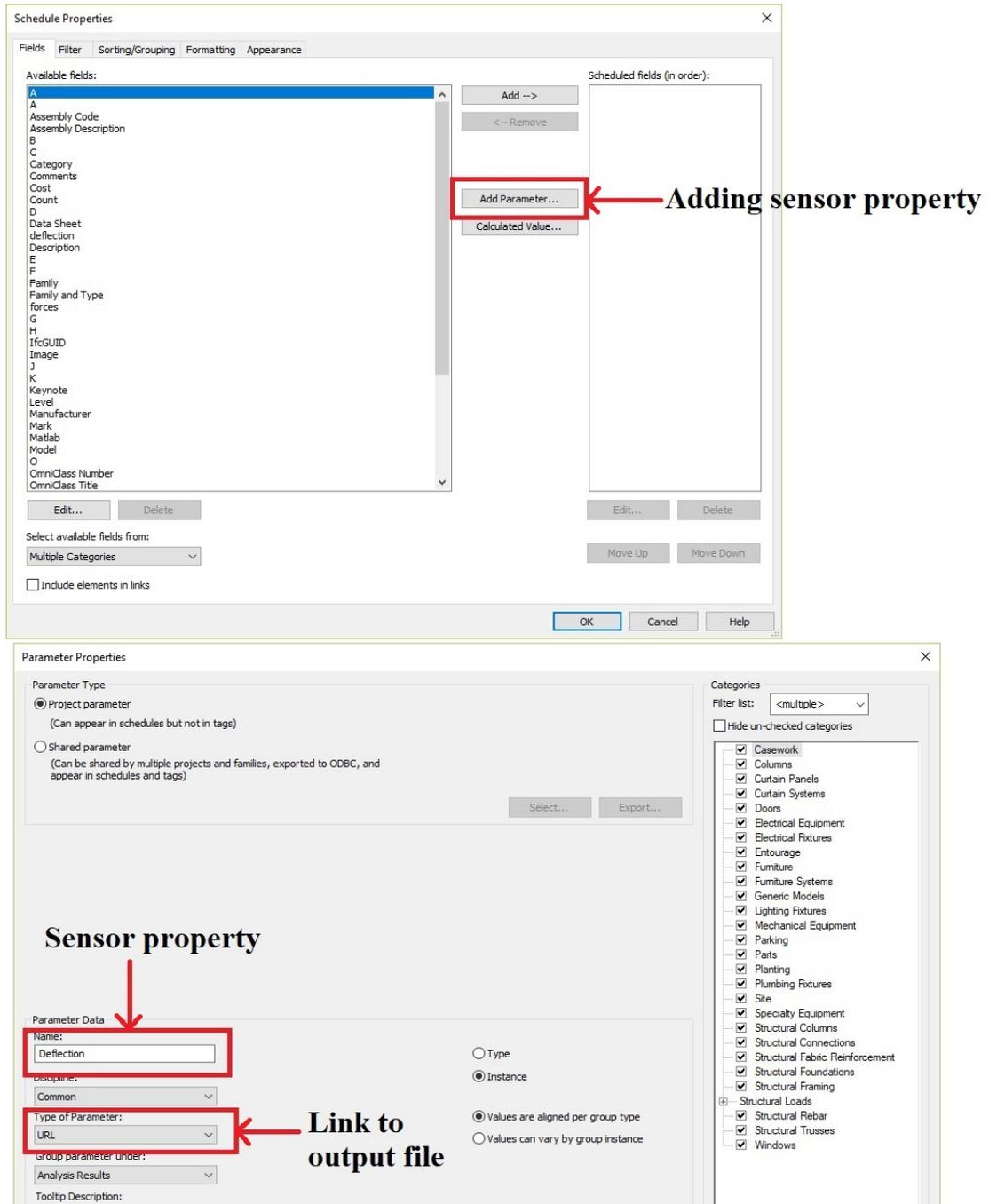
Figure 3.16: Sensor properties added to the Revit® model.
