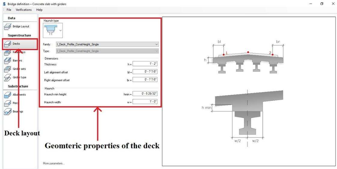
Figure 3.11: Deck layout of the bridge in Revit®.
