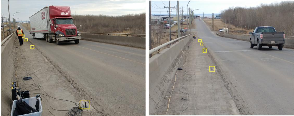
Figure 3.3: Sensors (highlighted using yellow box) placed on the side walk and the vehicles running on the bridge during the test.
