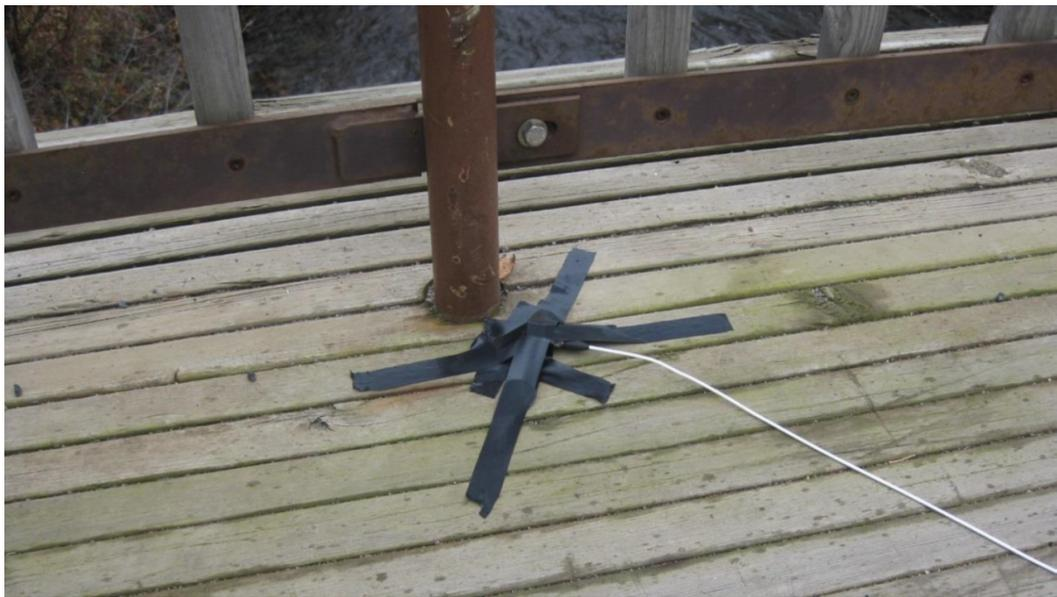
Figure 4.3: Typical sensor attached on bridge deck.
