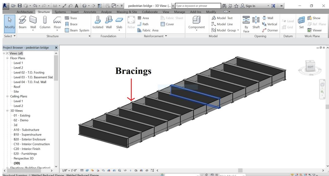
Figure 4.7: Design of bracing in BIM.
