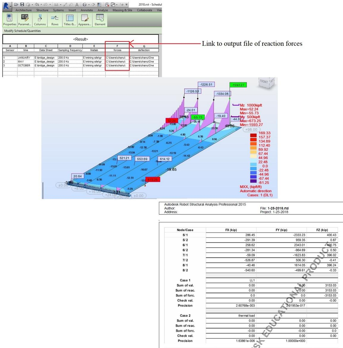
Figure 3.21: Report of the reaction forces obtained from the RSA®.
