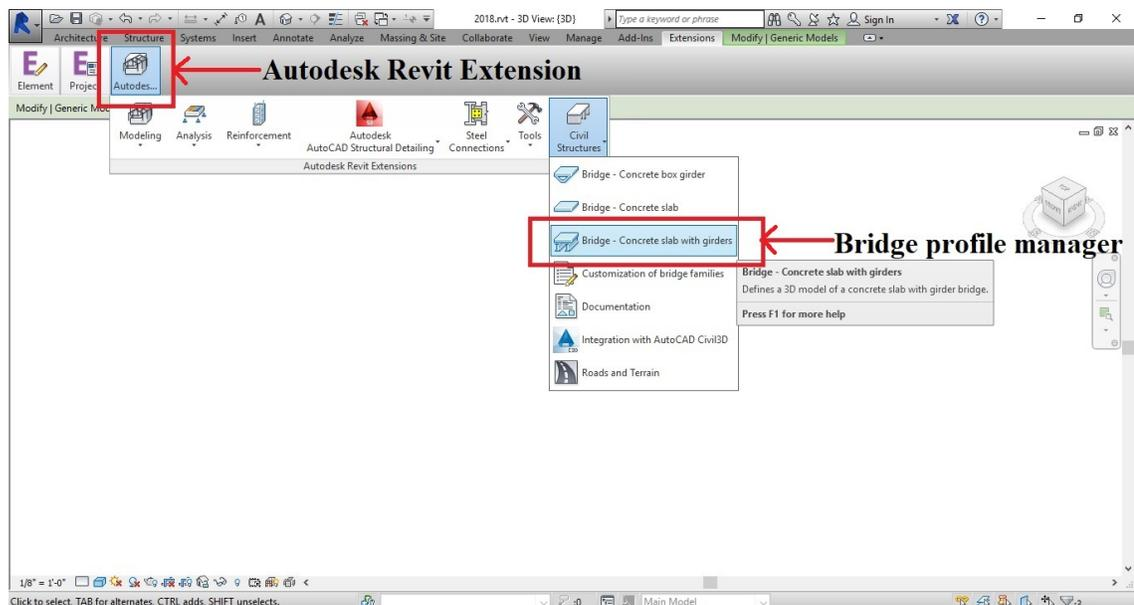
Figure 3.9: Autodesk bridge extension in Revit<sup>®</sup>.
