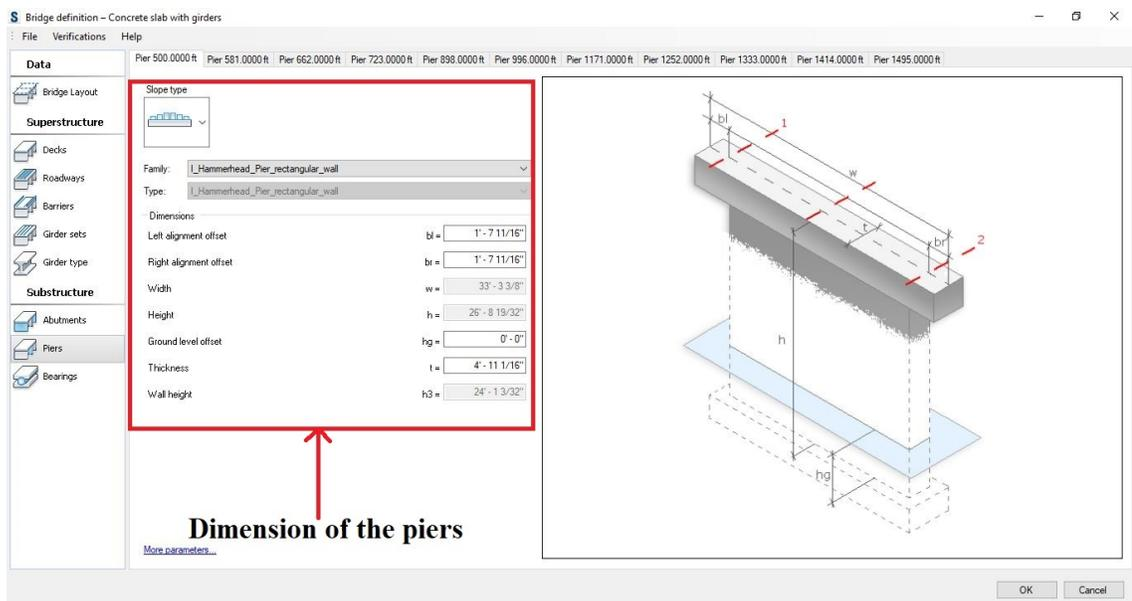
Figure 3.12: Alignment of piers of the bridge in Revit®.
