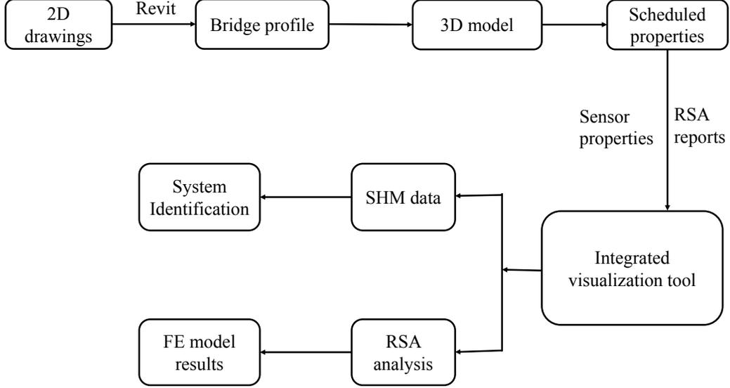
Figure 2.4: Detailed flowchart of the proposed integrated tool.
