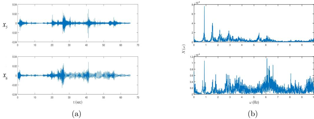
Figure 3.4: (a) Typical vibration data and (b) Fourier spectra of the measured data.
