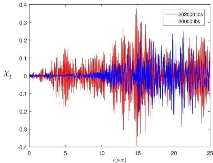
Figure 3.5: Time-history of mid-span sensor under maximum and minimum weights.
