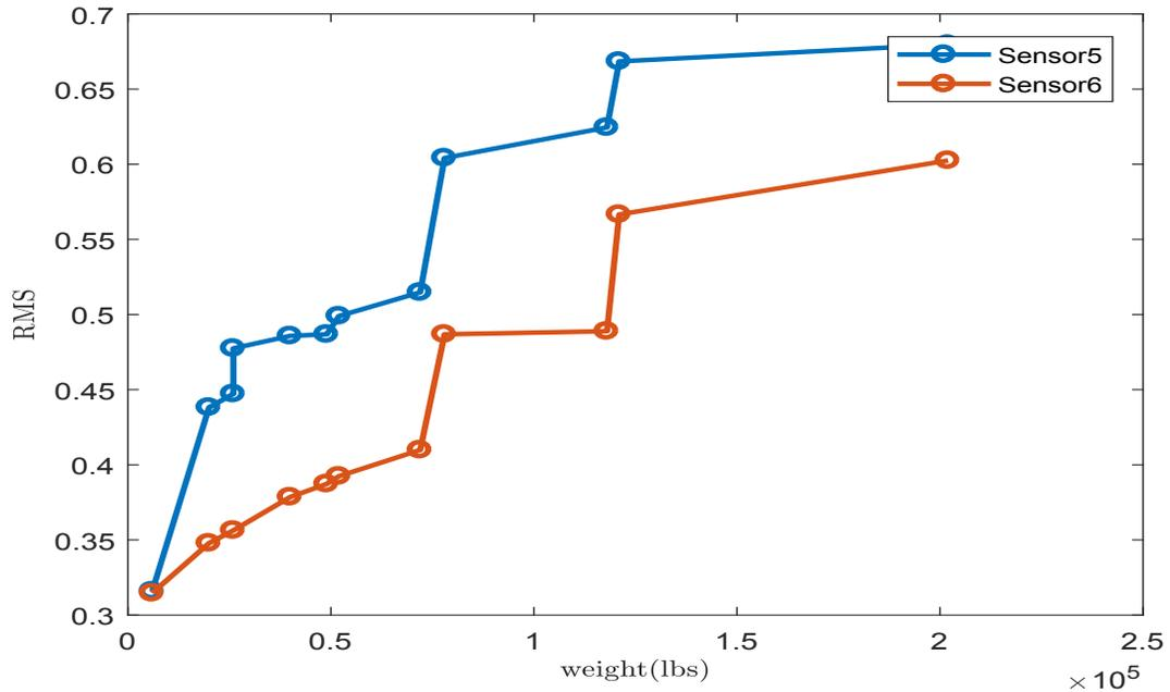
Figure 3.7: RMS acceleration of mid-span sensors under different traffic.
