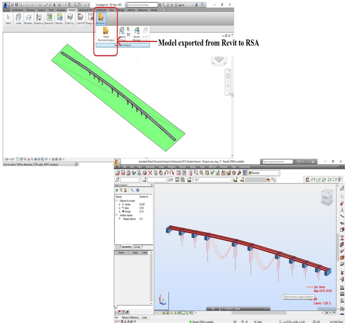
Figure 3.14: Transformation of the BIM model from Revit<sup>®</sup> to RSA<sup>®</sup>.
