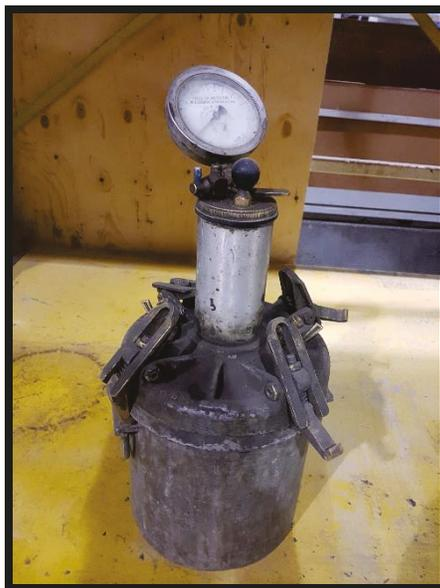
*Figure 6-6-2 Air Meter, Source: Primary*
