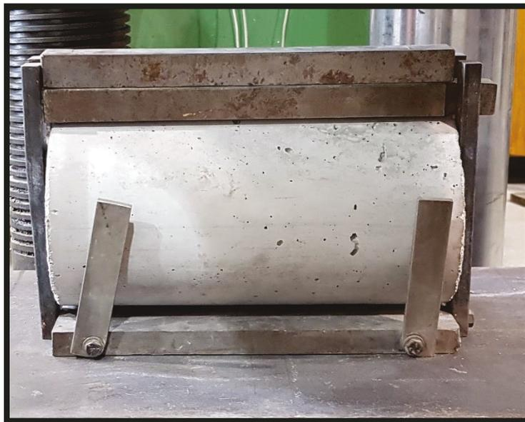
Figure 6-6-4 Splitting Tensile Jig, Source: Primary
