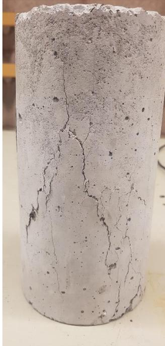
*Figure 8-1 Failed Compressive Strength Specimen, Source: Primary*
