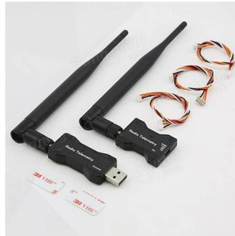
Figure 4.9: 3DR Telemetry Radio
