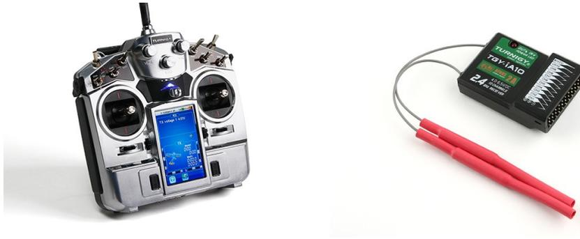
Figure 4.8: (a) RC Transmitter; (b) RC Receiver
