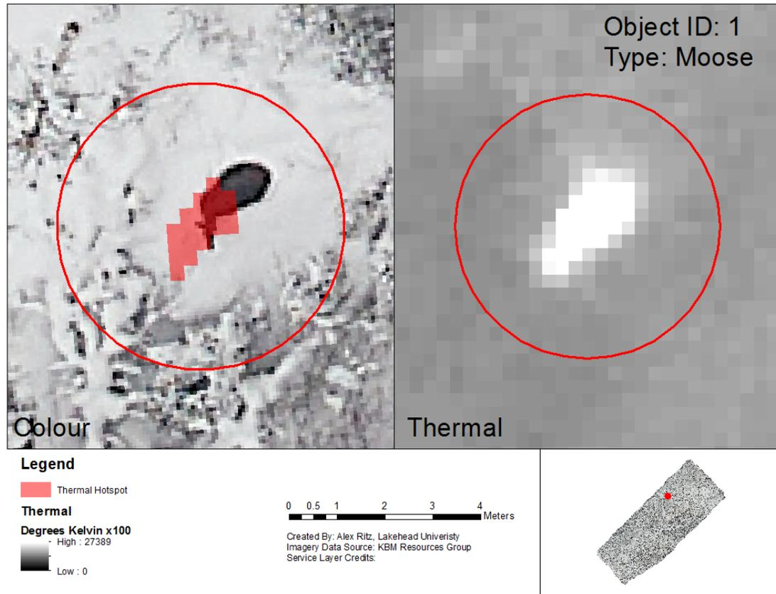
**Figure 4.3.2.** Example of colour (7.5 cm/pixel) and thermal (30 cm/pixel) imagery of moose thermal hotspot. Images taken on January 21, 2016 over La Verendrye Provincial Park, Ontario. Specific location within the imagery is depicted in the lower-right map. The thermal hotspot generated by automated model overlays moose in thermal and colour imagery.
