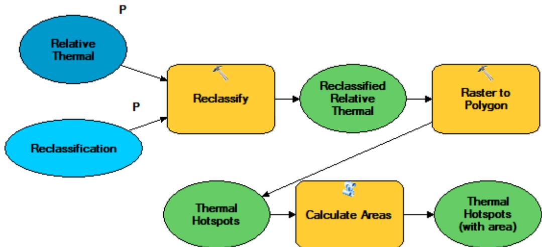
**Figure 4.2.3.** The second portion of the model uses the relative thermal raster created in Figure 4.2.2 to output thermal hotspot polygons with measured areas. Diagram symbology is as in Figure 4.2.2.
