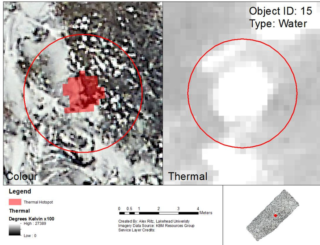
**Figure 4.3.3.** Example of a thermal hotspot of water incorrectly identified as moose. It is clear in the thermal imagery that the high thermal values are following a linear feature, and the colour imagery is clearly not a moose. Comparison with Figure 4.3.2 shows the clarity of moose in the colour imagery.
