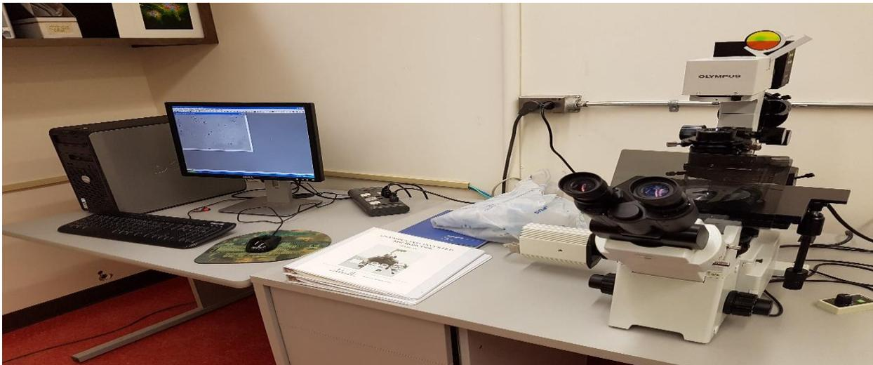
Figure 17: Olympus IX51 Inverted Microscope
