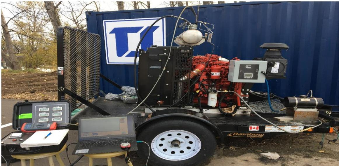
Figure 21: Cummins Engine Testing Setup
