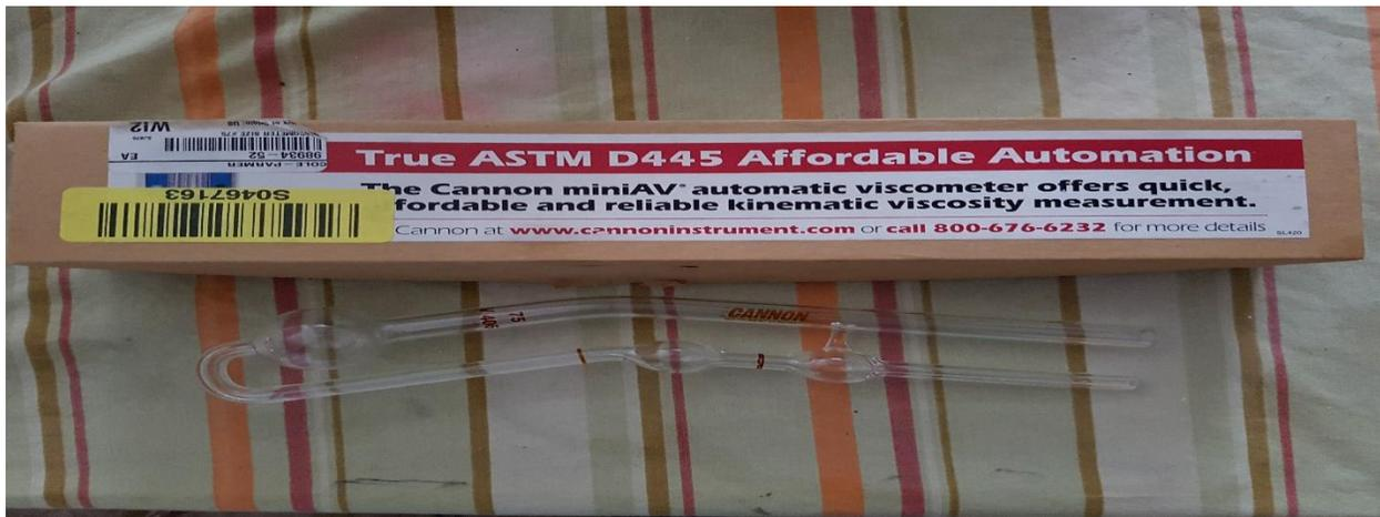
Figure 13: Kinematic Viscometer
