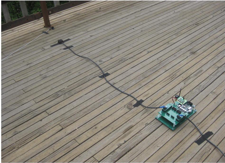
Figure 4.14: The Narada unit at the mid-span of the bridge
