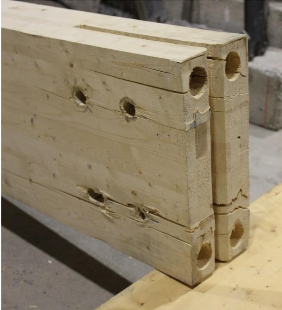
Figure 4.15 Brittle failure mode in Test 3B with four bolts and five-times bolt diameter end distance.
