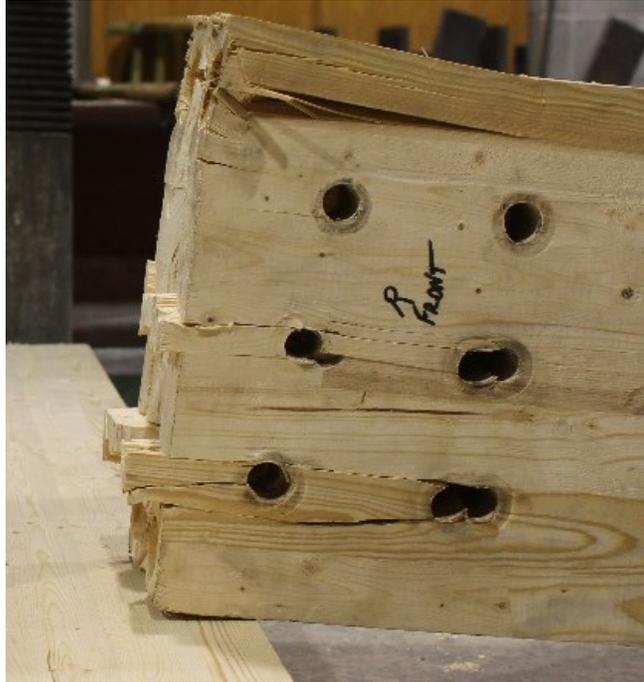
(a) Brittle failure modes in Test 2S with six bolts and four-times bolt diameter end distance.
