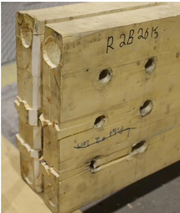
Figure 4.16 Brittle failure mode in Test 2B with six bolts and four-times bolt diameter end distance.
