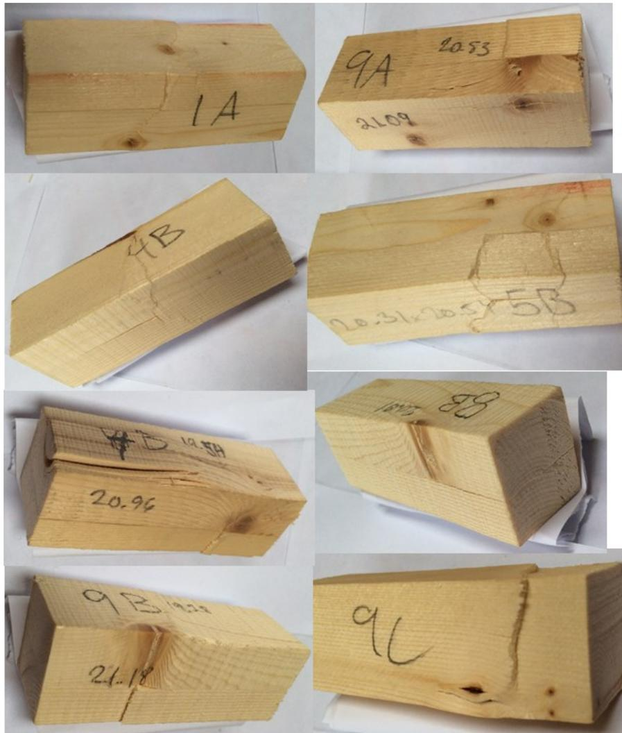
Figure 2.18 Compression stick samples from Groups A, B and C.
