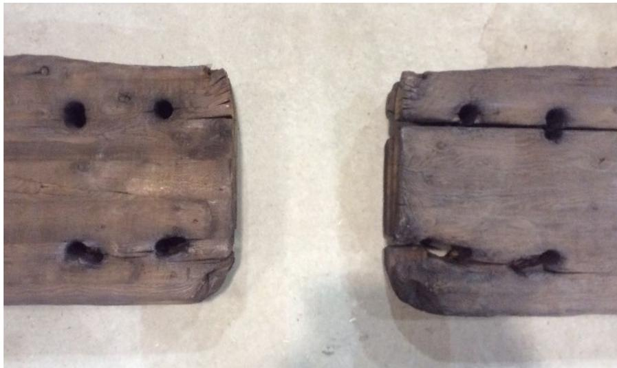
Figure 5.16 Glulam beam sections with the char layer removed, Test 1F
