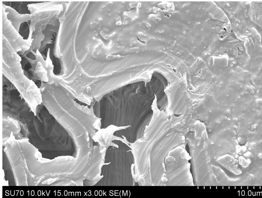
Figure 2.24 Glulam SEM cross section, glue-wood bond and interface details.
