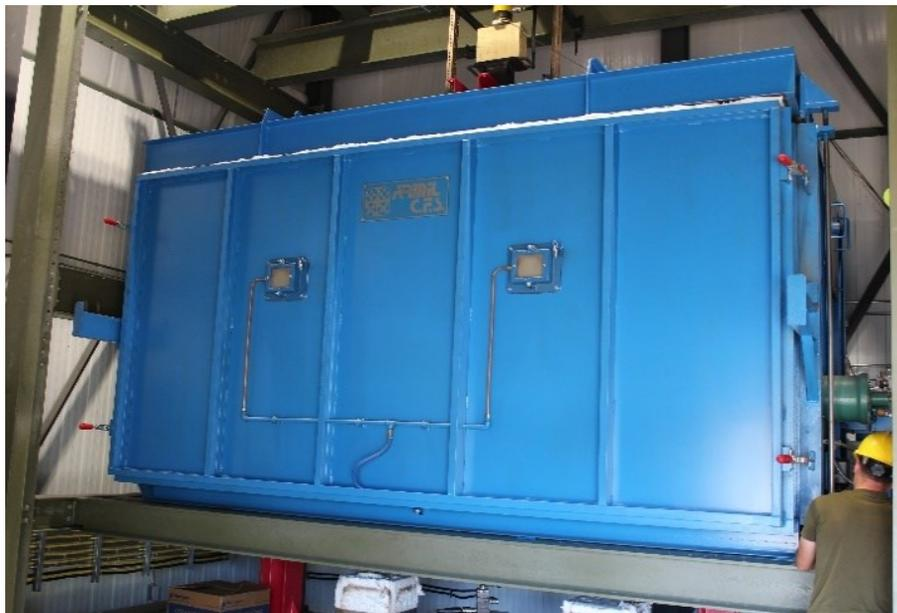
Figure 3.3 Large fire testing furnace accommodated at LUFTRL.
