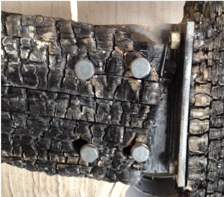
Figure 5.18 Failure modes observed in STS-strengthened connection with four bolts and five-times bolt diameter end distance (hole elongation, reduced brittle failure modes and complete combustion of almost all wood between the face and the first column of bolts)
