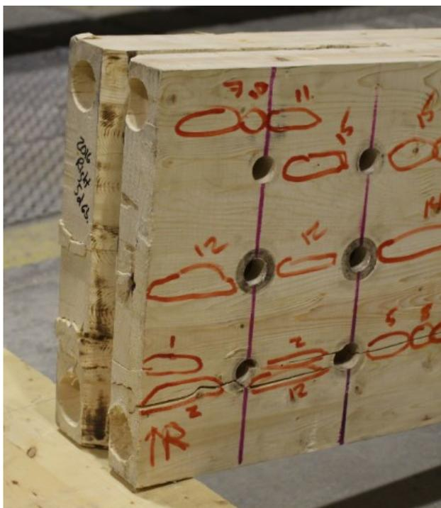
Figure 4.17 Brittle failure mode in Test 4B with six bolts and five-times bolt diameter end distance.
