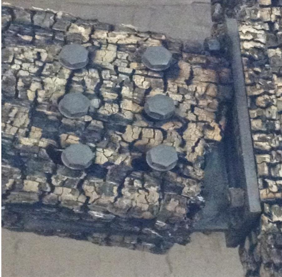
Figure 5.19 Failure modes observed in STS-strengthened connection with six bolts and four-times bolt diameter end distance (increased hole elongation and reduced brittle failure modes)
