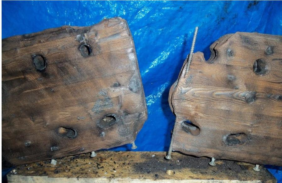
(c) Charred layer removed from Test 3FS assembly (four-bolt strengthened connections with five-times bolt diameter end distance).
