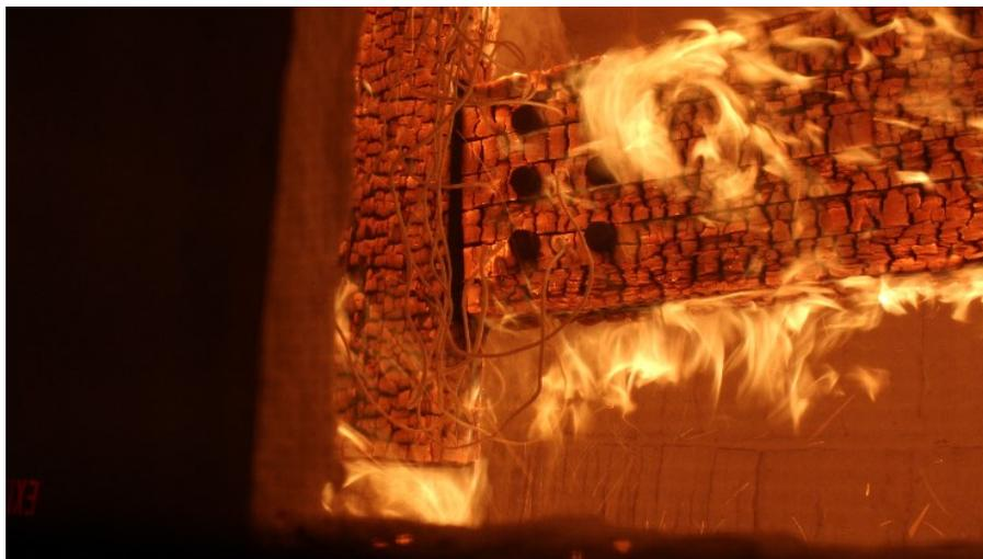
Figure 3.13 Beam-column test assembly with six bolts in three rows exposed to a standard fire.
