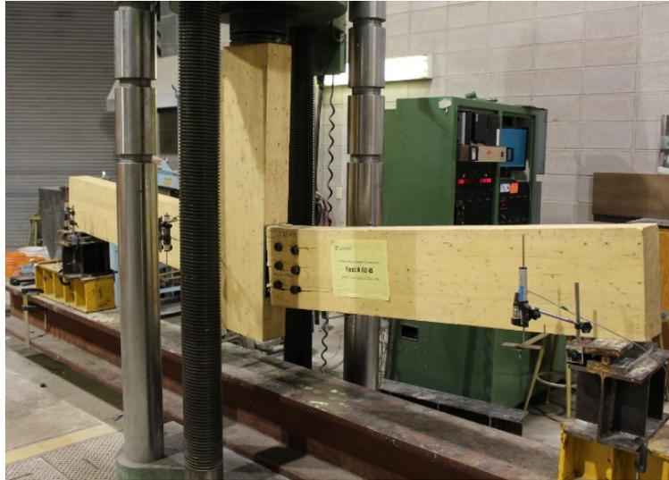
Figure 3.1 Lakehead University's UTM with glulam sample being loaded.
