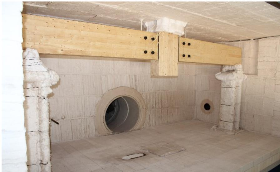
Figure 3.11 General beam-to-column test assembly inside the furnace with thermocouples and instrumentation installed.
