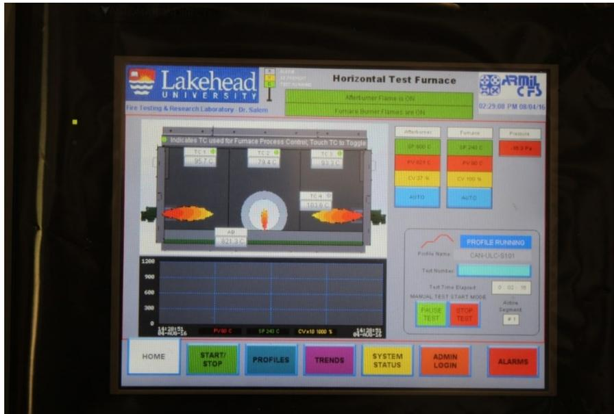
Figure 3.6 Human-Machine Interface (HMI) touch screen of the furnace’s control panel.
