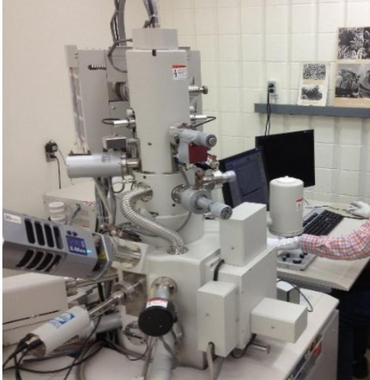
Figure 2.19 Hitachi Su-70 Schottky Field Emission SEM (Courtesy of Dr. Leitch, 2016).
