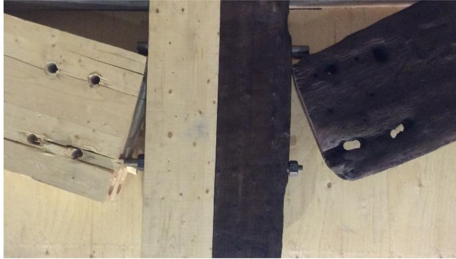
Figure 5.17 Row shear-out and splitting failure modes experienced in Test 1 and Test 1F assemblies at ambient and elevated temperatures, respectively
