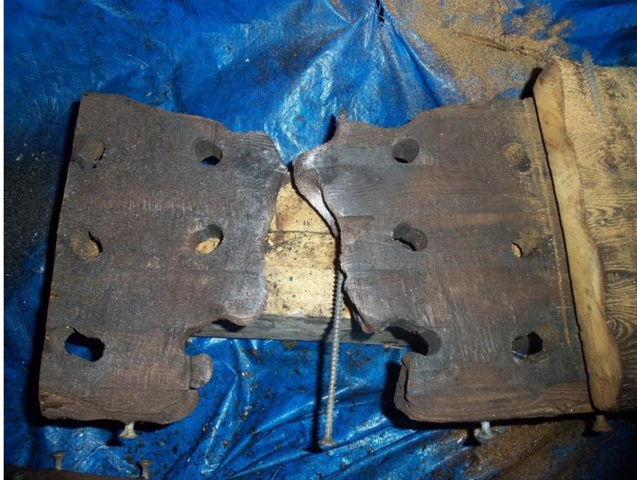
Figure 5.20 Thermally degraded cross section of the concealed slot cut of the strengthened connection with six bolts and five-times bolt diameter end distance,
