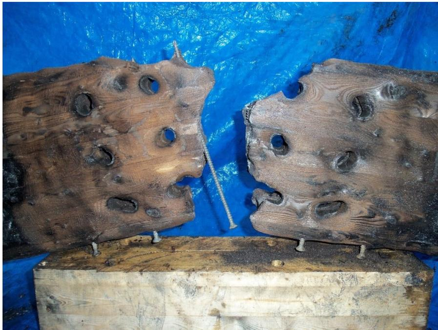
(d) Charred layer removed from Test 4FS assembly (six-bolt strengthened connections with five-times bolt diameter end distance).
