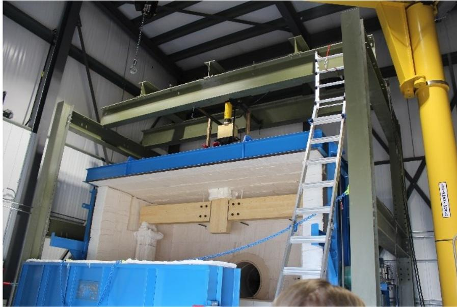
Figure 3.4 Fire testing furnace and steel loading frame.
