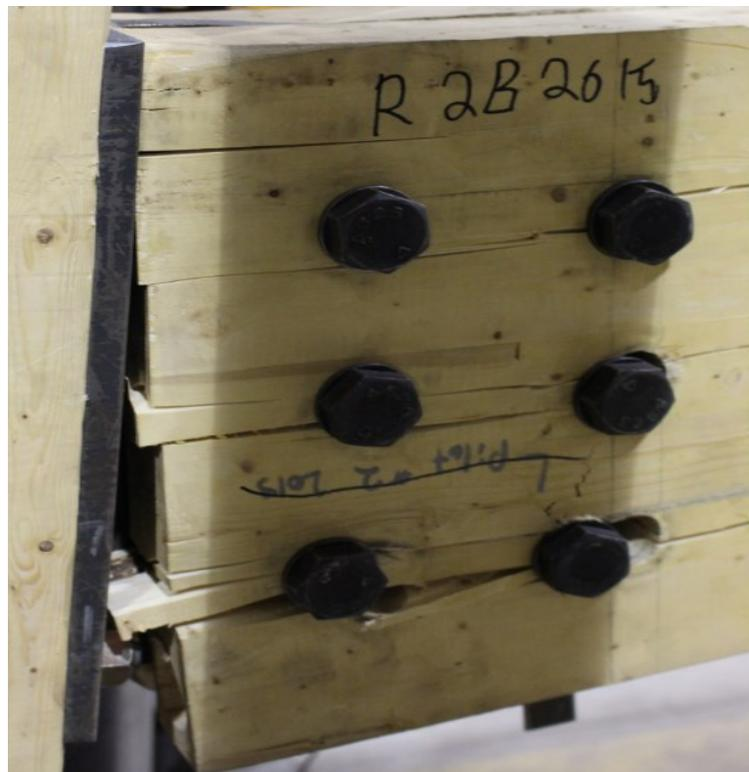
Figure 4.13 Typical observed glulam connection failure modes.
