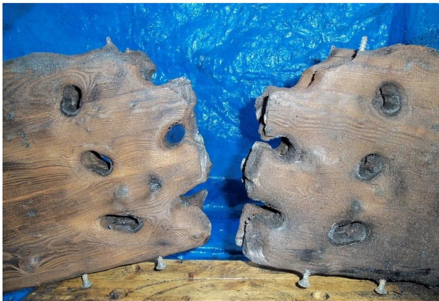
(b) Charred layer removed from Test 2FS assembly (six-bolt strengthened connections with four-times bolt diameter end distance).
