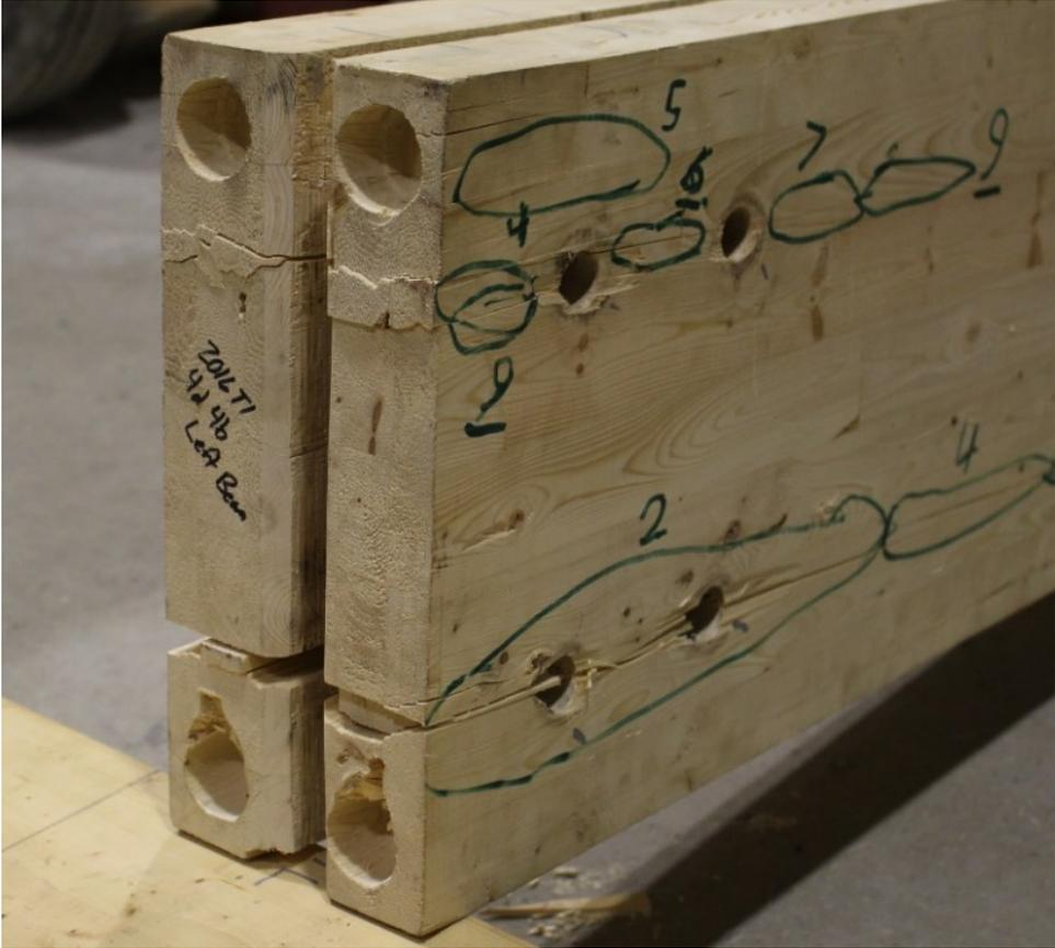
Figure 4.14 Brittle failure mode in Test 1B with four bolts and four-times bolt diameter end distance.
