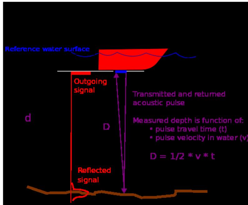
Figure 6.1.1.1. : Schematic of how depth is calculated using a single beam echo sounder (from Army Core of Engineers).
