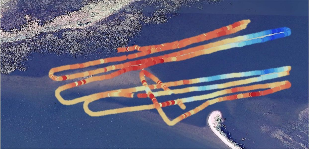
*Figure 5.1.1.3. Tracks of data points (depth measurements) collected near the mouth of Frog Portage, on Dog Lake. Colour coding of the data points reflect depth changes (Red reflects a shallower water column, while Blue represent a deeper area).*
