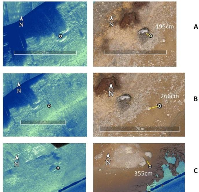
Figure 5.1.2.8. Comparison of spatial accuracy between the side scan sonar, and imagery captured with the UAV at the Hawk Bay Site.
