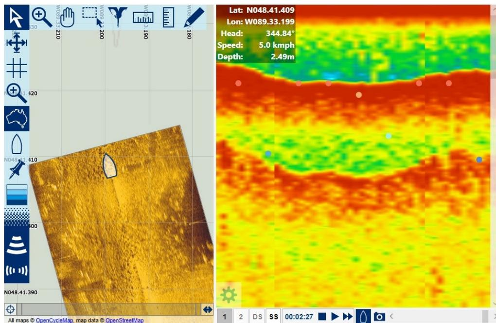
Figure 6.1.1.5. Right) Echogram of track R0091 shows that some of the depth returns are at odds with the bottom profile. Left) Side scan image (sonogram) of the R0091 track detecting the field of rocks and cobble below the transducer.
