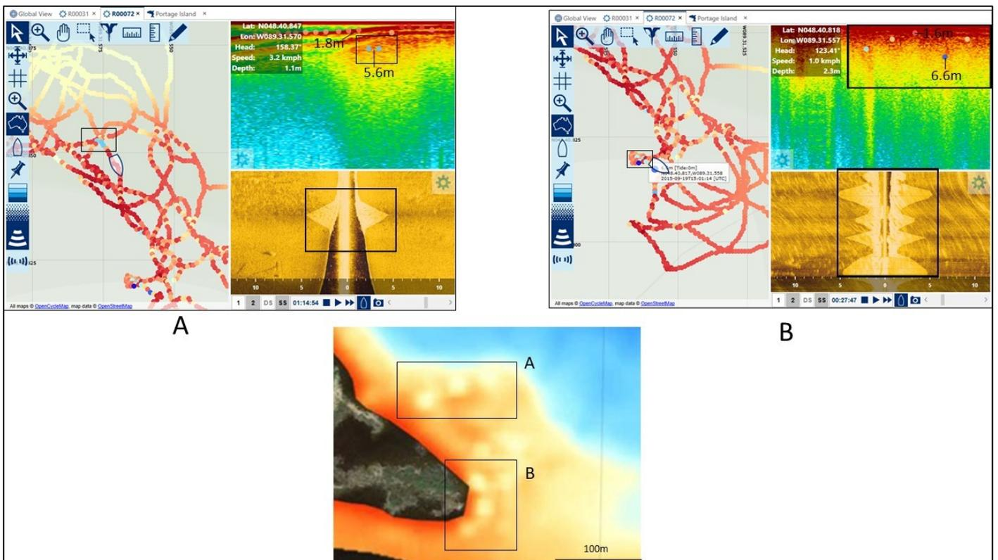
Figure 6.1.1.6. Anomalies in the bathymetric output (areas A and B) are compared to the sonograms taken from the same area. Evidence suggests human error caused the anomalies.
