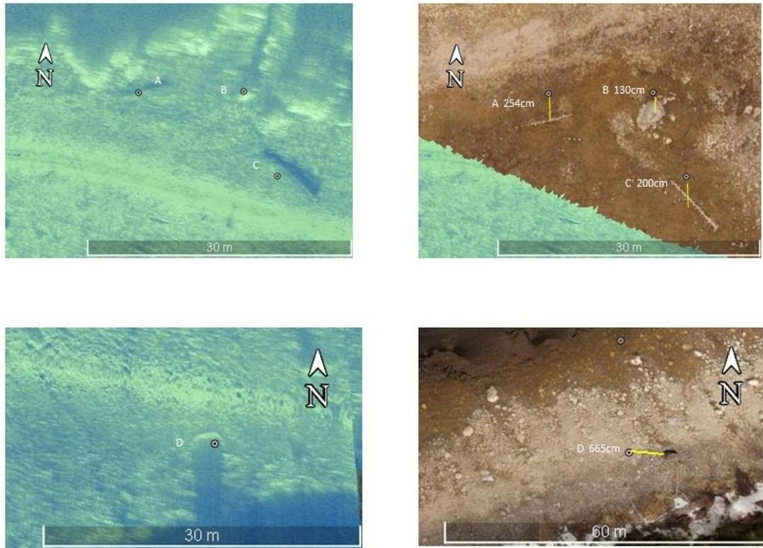
Figure 5.2.3.8. Comparison of spatial accuracy between the side scan sonar, and imagery captured with the UAV at the Portage Island Site.
