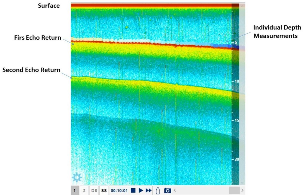
Figure 6.1.1.2. Schematic representing the different traits of an echogram.
