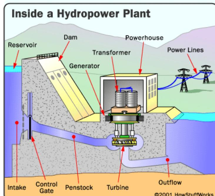
Figure 3.1.1. Schematic highlighting the many components of a Hydroelectric plant (borrowed from Castaldi *et al.*, 2003).
