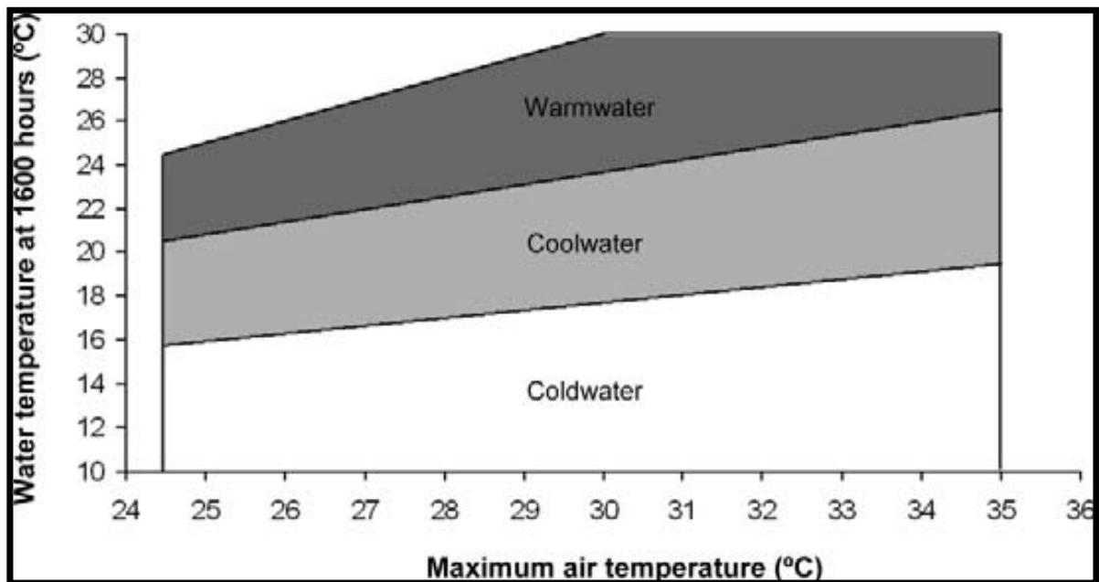
Figure 2.1: Re-print of Stoneman and Jone's (1996) nomogram of the maximum air and water temperatures at 1600 hours, used to estimate the thermal classification of stream sites from measurements of the daily maximum air temperature ( $\geq 24.58^{\circ}\text{C}$ ) and water temperature. (Source: Chu et al., 2009).
