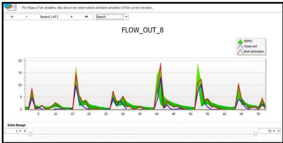
**Figure 5.2: 95ppu plot. The green area contains the 95% of predictive uncertainty corresponding to the behavioural parameter sets. The blue line represents observed flow data, while the red line shows the best simulation of the current iteration.**
