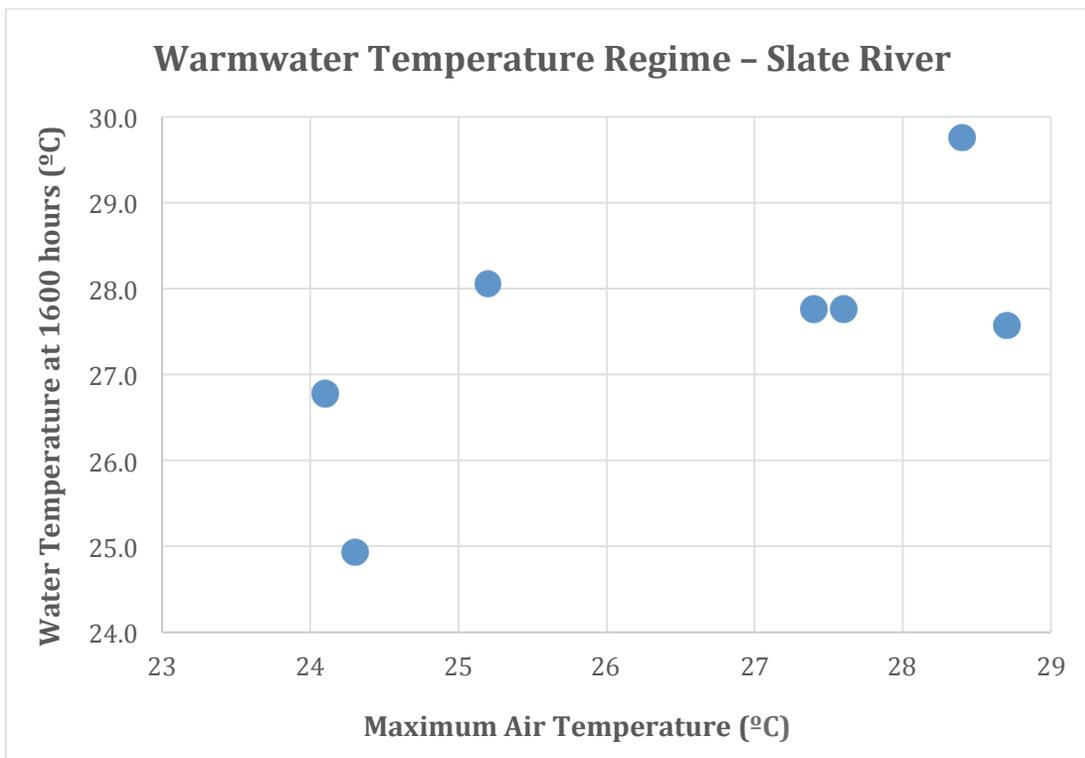
Figure 5.1a: Stream temperatures recorded when there was at least three consecutive days of air temperatures  $\geq 24.5^{\circ}\text{C}$ . Referring to Stoneman and Jones' nomogram, the data suggests that the Slate River is clearly a warmwater classification as the lowest water temperature exceeds the warmwater classification threshold.
