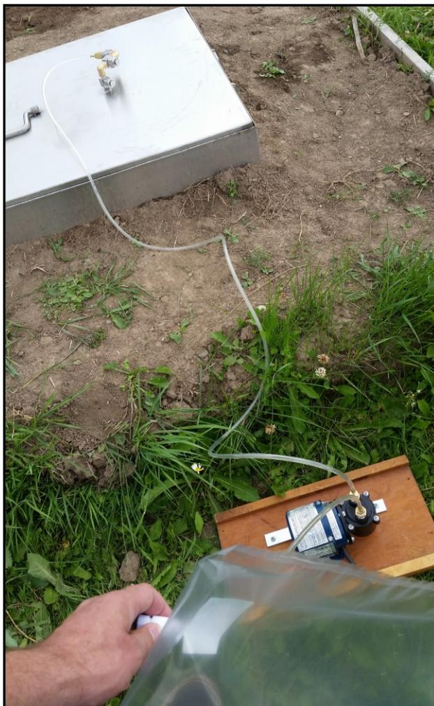
**Figure 5.2:** Vacuum pump draws a sample from the sealed static gas chamber.
