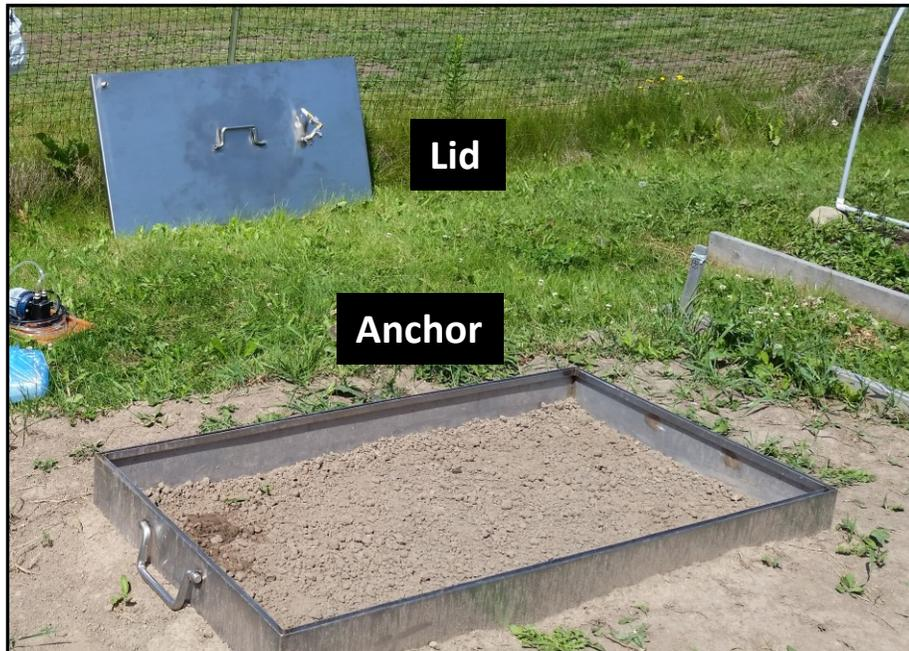
**Figure 5.1:** The installed static gas chamber.
