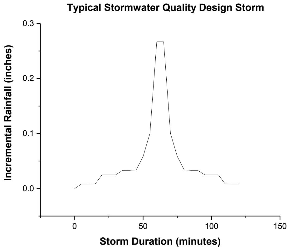
**Figure 7.** Stormwater Quality Design Storm based on precipitation rate of 1.25"/2 hrs. (Blick et al., 2004)
