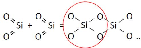
**Figure 2-1: SiO<sub>2</sub> bonding within quartz to form SiO<sub>4</sub>.**
