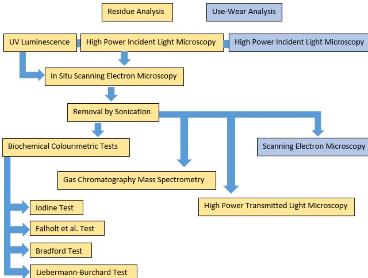
**Figure 4-3: Multi-analytical approach to residue and use-wear analysis.**
