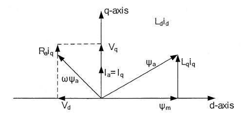
Fig 2.4 Phasor diagram of a IPMSM with  $i_d = 0$ .
