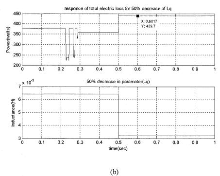
Fig.3.7 Simulated total loss for IPMSM drive while parameter  $L_q$  changes: (a) proposed loss minimization algorithm (b)  $i_d$ =0.
