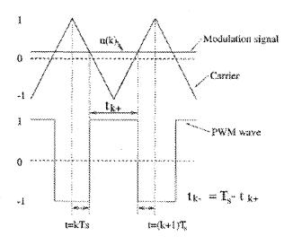
Fig. 2.6 Two level carrier based-PWM.
