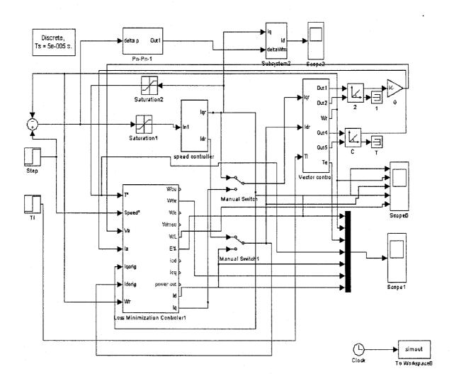
Appendix B.3 Complete Loss Minimization Model with Field oriented PM control.
