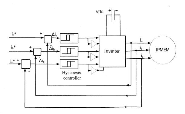
Fig. 2.9 Block diagram of current controlled voltage source inverter.
