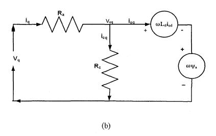
Fig.3.1 d- q axis model of IPMSM incorporating iron loss.
