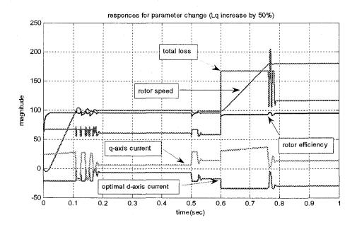
Fig. 3.8 Simulated speed, efficiency, total loss and currents responses for IPSM drive with the proposed loss minimization algorithm.
