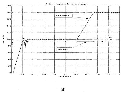
Fig. 3.4 Simulated responses of the proposed loss minimization based IPMSM drive; (a) speed, (b)  $i_q$ , (c)  $i_d$  and (d) efficiency.
