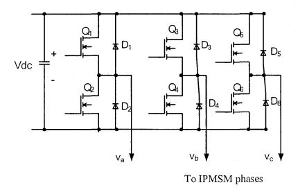
Fig. 2.8 Three half-bridge inverter.
