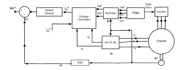
Fig.2.3 Vector control of electric motors.
