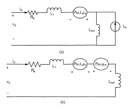
Fig.2.1 d-q axis equivalent circuit model of IPMSM; (a) d-axis and (b) q-axis.
