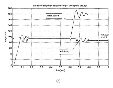
Fig. 3.5 Simulated responses of IPMSM drive with  $i_d$ =0 control technique; (a) speed, (b) $i_q$ , (c)  $i_d$  and (d) efficiency.
