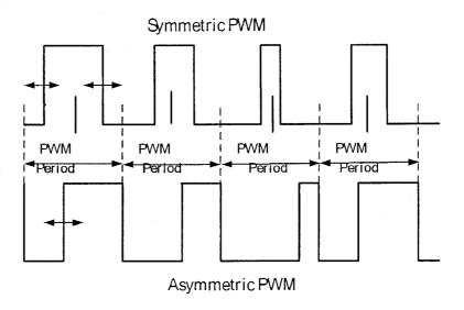
Fig.2.5 Symmetric and asymmetric PWM signals.
