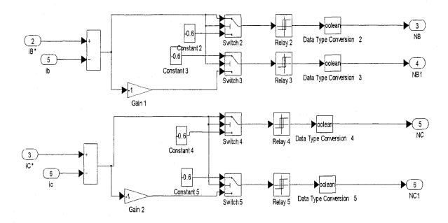
Appendix B.9 Real time Current controller and PWM signal generator.
