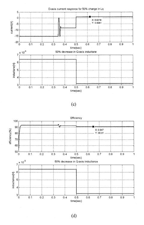
Fig.3.6 Simulated responses of IPMSM drive with parameter change for proposed loss minimization algorithm: (a) speed, (b) $i_q$ , (c)  $i_d$  and (d) efficiency.
