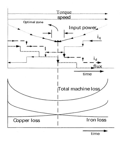
Fig. 3.2 An illustration of efficiency optimization control principle with d-axis current decrement.
