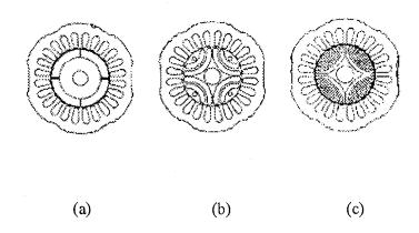
Fig. 1 Show the cross-section of (a) SMPMSM, (b) IPMSM and (c) SyncRM rotor configuration.
