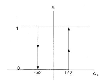
Fig. 2.7 Input-output characteristic of hysteresis current controller.
