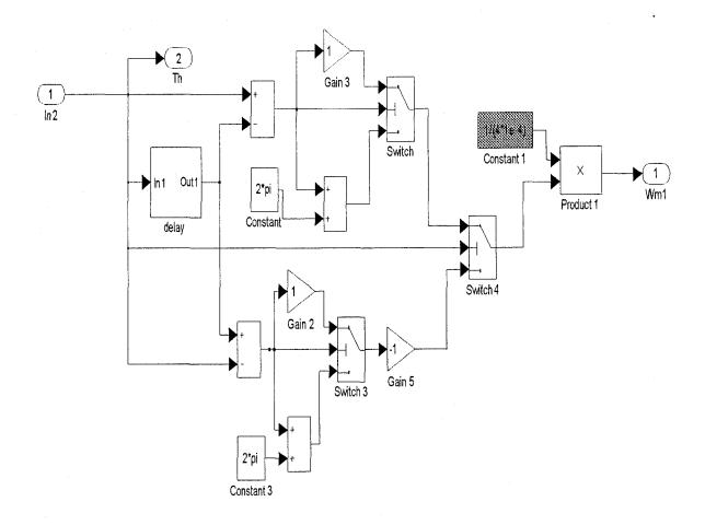
Appendix B.8 Speed calculator from the encoder position input.
