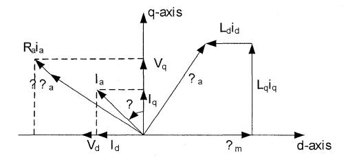
Fig.2.2 Basic phasor diagram of an IPMSM.
