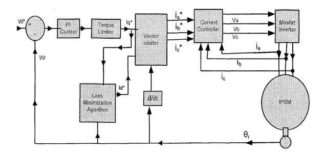
Fig.3.3 Block diagram of the proposed loss model based efficiency optimization of IPMSM drive.
