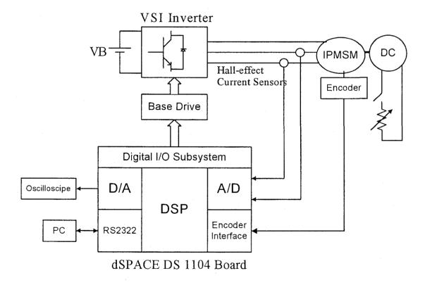
Fig. 4.1 Block diagram of the hardware schematic of the VSI-fed IPMSM drive.
