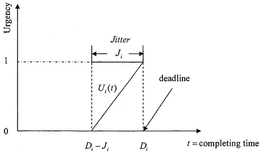
Figure 4.2 Concept of jitter for RT traffic
