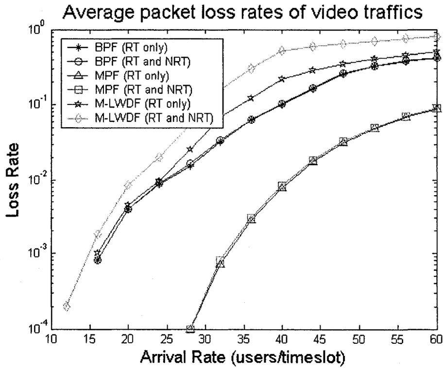
Figure 5.13 Average packet loss rates of video traffics with RT traffic only and RT and NRT traffics together
