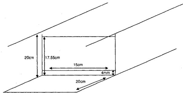
Figure 9 - Dimensions of a compartment within the flow through aquarium. Each compartment housed a breeding pair of fathead minnows and a spawning substrate (modified from Hardy 2002).
