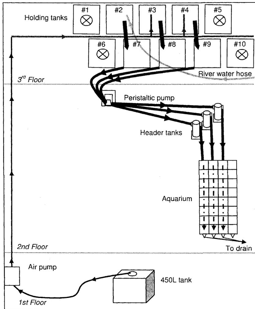
Figure 5 – Diagram of the bioassay setup at AbitibiBowater - Thunder Bay.
