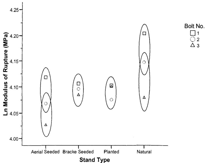
Figure 20. Mean natural log of modulus of rupture for each bolt position categorized by regeneration method. Markers found within the same ellipses signify bolts within each regeneration method that were not significantly different in MOR. Bolts 1, 2 and 3 were located at approximately 1, 2 and 4 m from the base of each tree.
