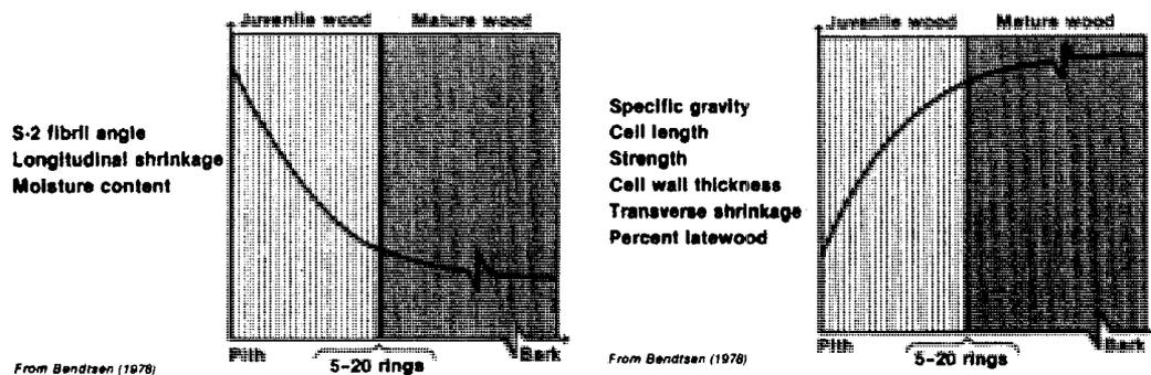
Figure 4. Schematic diagrams of wood property changes from juvenile to mature wood (Bowyer *et al.* 2003).
