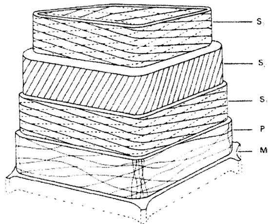
Figure 2. A three dimensional illustration of cell wall layers and associated microfibril angles. ML- middle lamella; P – primary wall; S – secondary wall subdivided into corresponding layers (Wilson and White 1980).
