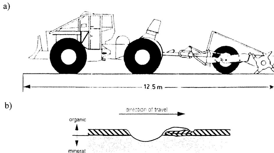
Figure 1. a) Illustration of the standard Bräcke configuration (Van Damme *et al.* 1988); b) cross-sectional view of a Bräcke scalp (Sutherland and Foreman 1995).
