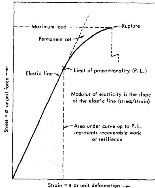
Figure 7. Typical stress-strain diagram for static bending to failure (Panshin and de Zeeuw 1980).
