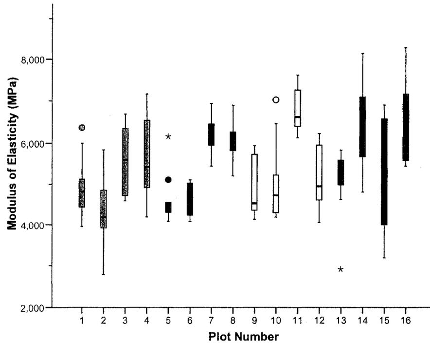
Figure 15. Comparative boxplots of modulus of elasticity for each plot. Aerial seeded: plots 1 – 4; Bräcke seeded: 5 – 8; planted: 9 – 12; natural: 13 – 16.
