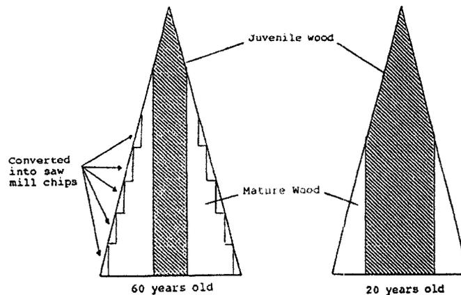
Figure 6. An illustration demonstrating the varying portions of juvenile wood with respect to tree age and the associated amount of mature wood (Zobel and Sprague 1998).
