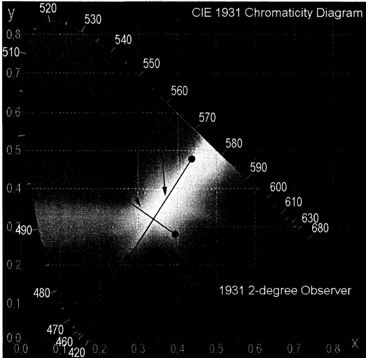
*Chromatic Properties of B/Y and R/G Stimuli. Chromatic contrast modulation was defined along the two axes that connect the B/Y and R/G peak-to-trough endpoints.*
