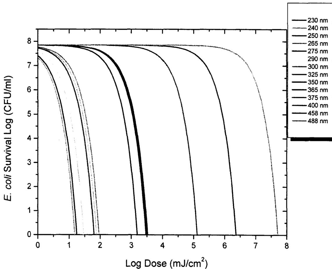
Figure 2. 20 - Best fit curves of all *E. coli* survival vs. dose wavelengths between 230 to 488 nm. The visible wavelengths 514 nm and 532 nm were not included because there was no kill observed at these wavelengths.
