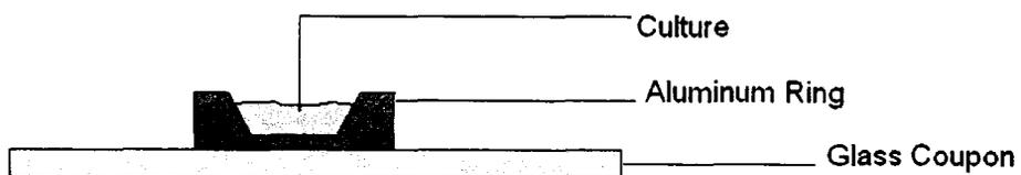
Figure 2. 3 - Sample holder used for UV radiation in planar and lateral views.
