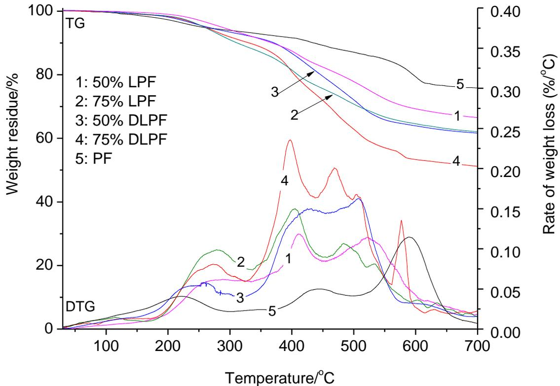
**Figure 7-4.** TG and DTG profiles of OLPF, DLPF and PF resins.
