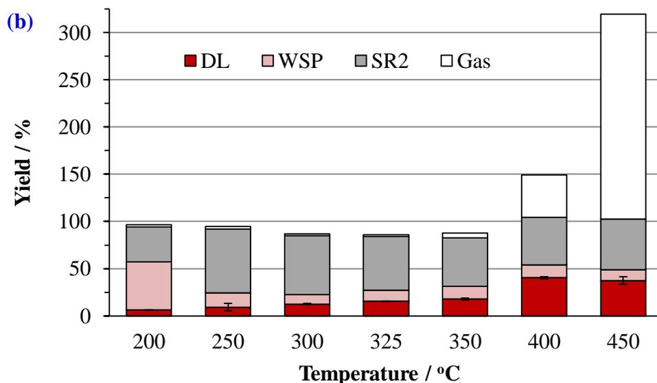
**Figure 6-3.** Effects of reaction temperature on the yields of DL, WSP, SR<sub>2</sub> and gas products obtained in 50/50 (v/v) water-ethanol (a) and in pure ethanol (b) for 2 hr.
