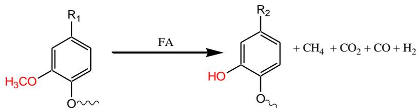
**Figure 8-4.** A possible cleavage pathway of methoxyl group on lignin polymer (FA: Formic acid).
