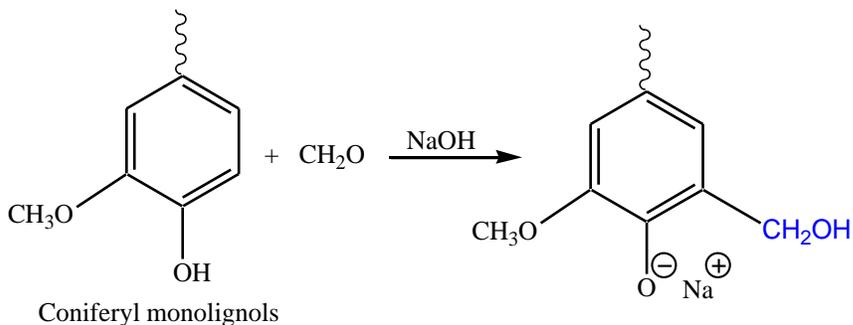
**Scheme 5-2.** Methylation reaction mechanism of bio-oil with formaldehyde.
