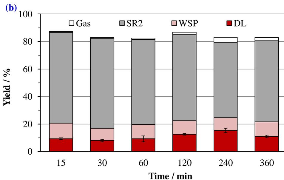
**Figure 6-2.** Effects of reaction time on yields and distribution of the lignin degradation products in 50/50 (v/v) water-ethanol (a) and in pure ethanol (b) at 300 °C in a 14 mL micro reactor.
