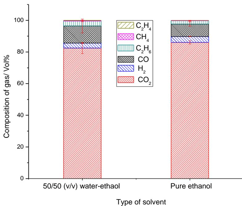
**Figure 8-1.** Composition of gas products produced from all the runs shown in Table 8-1.
