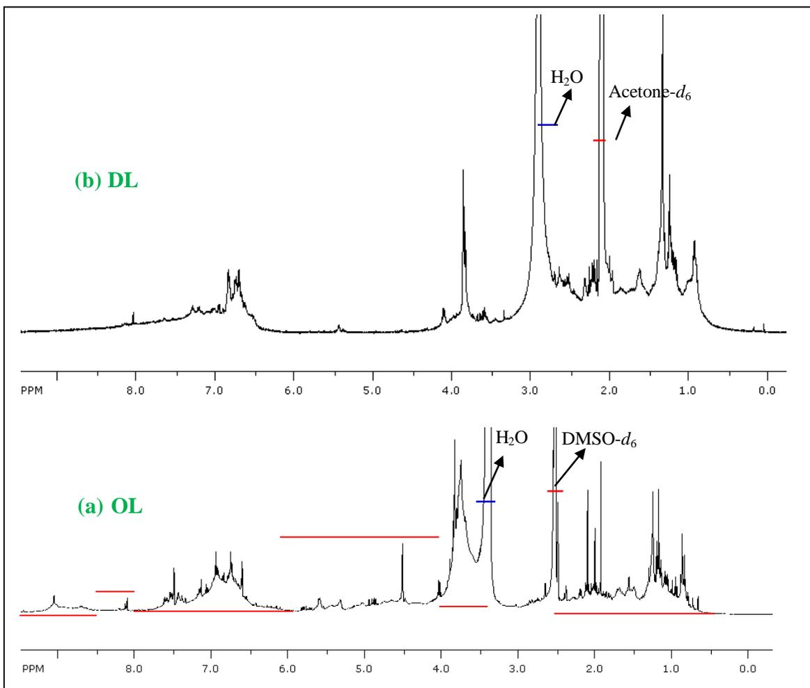
**Figure 8-6.** <sup>1</sup>H NMR spectra of OL (a), and DL (b). OL in DMSO-*d*<sub>6</sub>. DL (350 °C, formic acid, 2 hr, 50/50 (v/v) water-ethanol) in Acetone-*d*<sub>6</sub>. Peak at 2.08 ppm, 2.5 ppm and 3.3 ppm are derived from Acetone-*d*<sub>6</sub>, DMSO-*d*<sub>6</sub> and residue moisture in sample, respectively.
