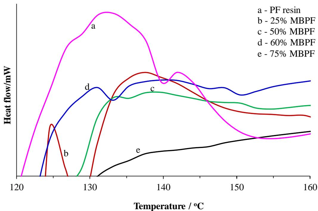
**Figure 5-5.** DSC curves for different resin systems obtained at a heating rate of 5 °C/min from 40 °C to 250 °C with 50 mL/min of N<sub>2</sub>.
