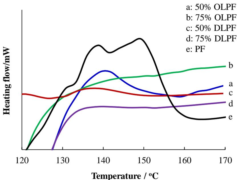
**Figure 7-3.** DSC curves of OLPFs, DLPFs and PF.
