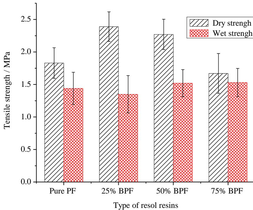
**Figure 4-6.** Tensile strength of the plywood samples bonded with the BPF and PF resol resins (Dry strength: test after conditioning; Wet strength: test after boiling in water for 3h).
