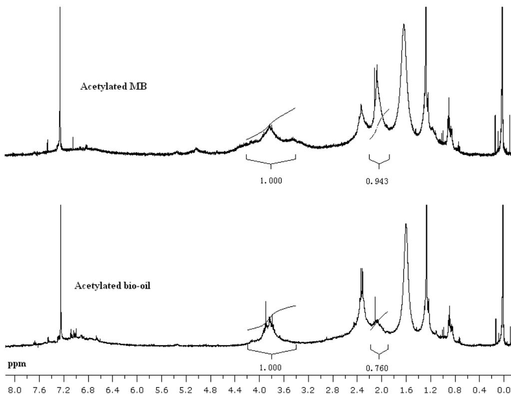
**Figure 5-1.**  $^1\text{H}$  NMR spectrum of the acetylated raw bio-oil and the acetylated methylolated bio-oil. Peak at 7.26 and 1.6 ppm are the solvent and water, respectively.
