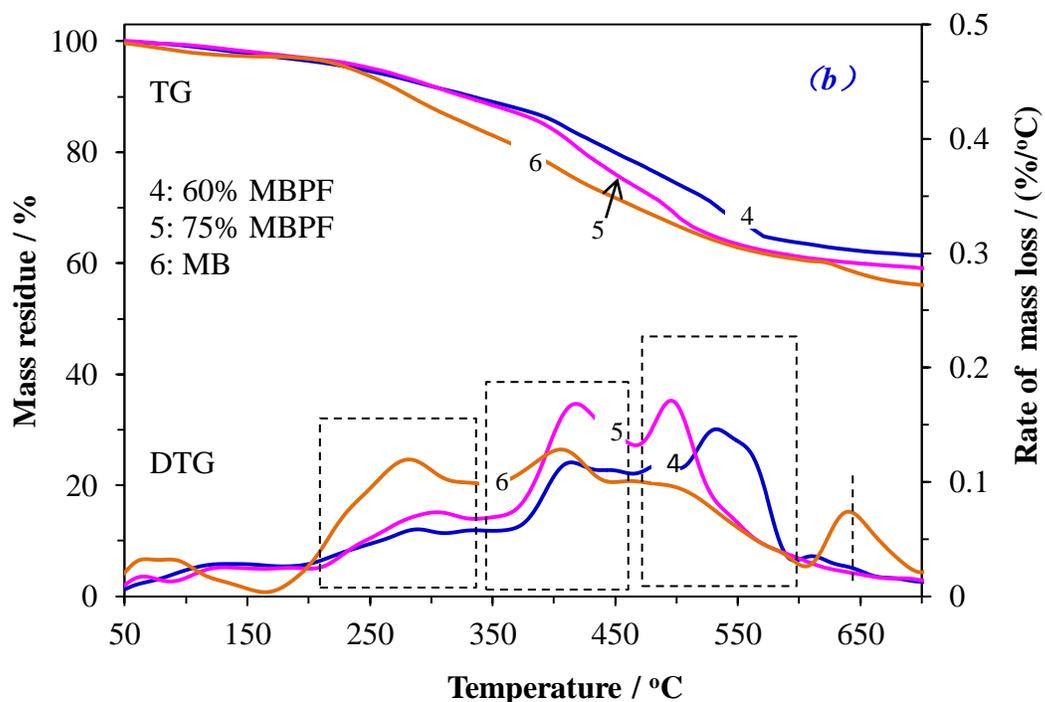
**Figure 5-6.** TG and DTG profiles of various MBPF resins obtained by heating from 25 to 700 °C in 30 mL/min of N<sub>2</sub> atmosphere.
