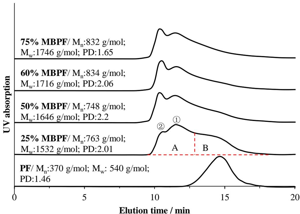
**Figure 5-4.** GPC chromatograms of MB and MBPF resins.
