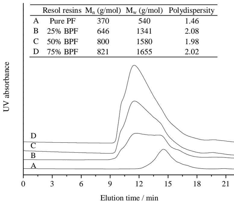
**Figure 4-5.** GPC chromatograms of the acetylated BPF and PF resole resins (using THF as the eluent at 1 mL/min, UV detector at 270 nm, polystyrene standards).
