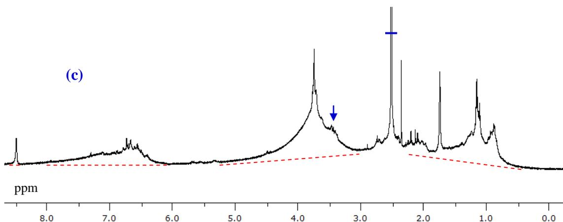
**Figure 6-5.**  $^1\text{H}$  NMR spectra of the original AL (a) and the DL obtained at 300 °C in 50/50 (v/v) water-ethanol for 2 hr without (b) and with Ni10/AC catalyst (c). The big peak at 2.5 ppm and 3.3 ppm is derived from the solvent and residual moisture in the AL, respectively.
