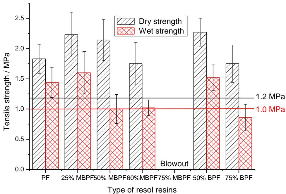
**Figure 5-7.** Tensile strength (dry and wet) of the plywood specimens bonded with MBPF and PF adhesives.
