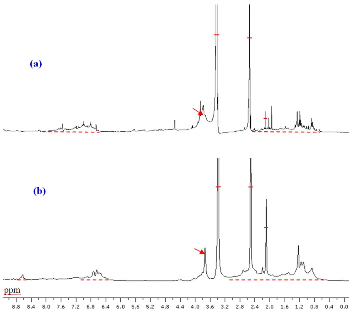
**Figure 7-1.**  $^1\text{H}$  NMR spectra of original OL (a) and DL (b) which was obtained at 340 °C for 2 hr with Ni10/AC in 50/50 (v/v) water-ethanol using the 1 L stirred autoclave reactor.
