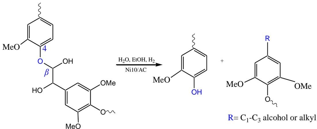
**Figure 7-2.** A typical hydrogenolysis/hydrolysis cleavage of  $\beta$ -O-4 linkage.
