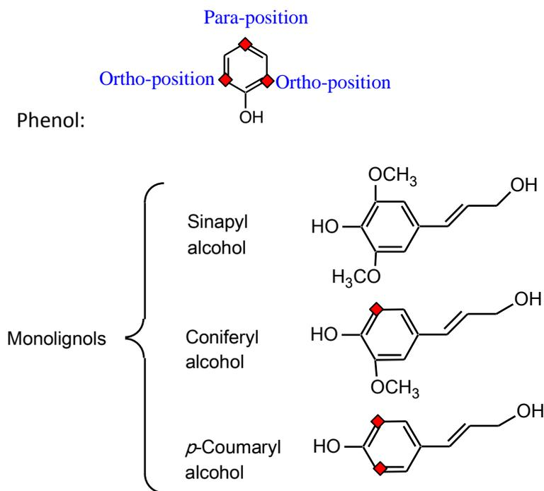
**Scheme 5-1.** Reactive sites in phenol and three monolignols for PF resin synthesis reactions.
