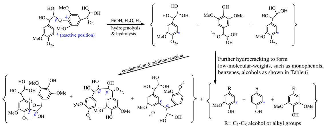
**Figure 6-6.** Possible lignin hydrothermal degradation mechanism in 50/50 (v/v) water-ethanol co-solvent under hydrogen.
