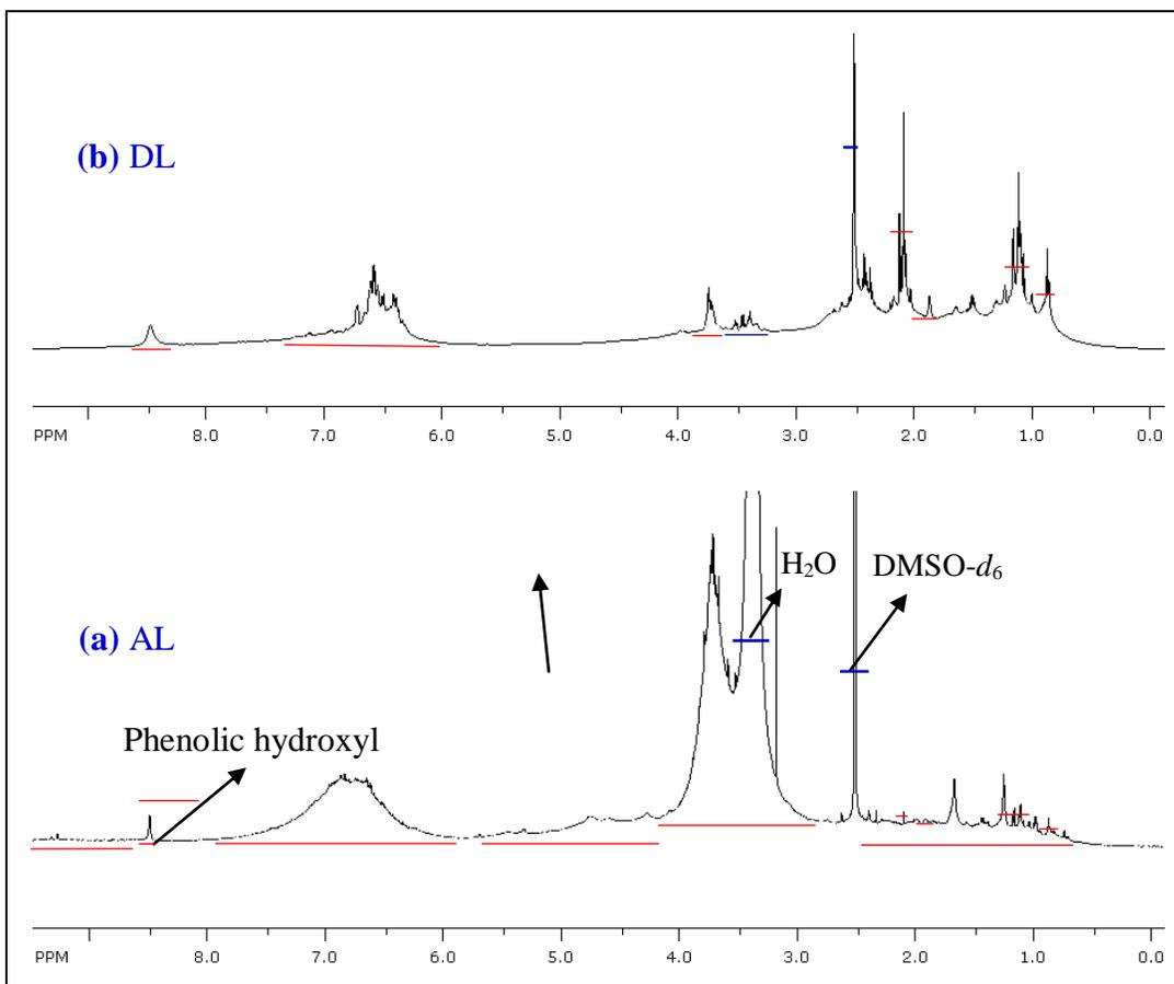
**Figure 8-3.**  $^1\text{H}$  NMR spectra of AL (a) and DL (b) in  $\text{DMSO-}d_6$ . DL was produced from the case in 50/50 (v/v) water-ethanol together with formic acid. Peak at 2.5 ppm is derived from the solvent. Peak at 3.3 ppm is derived from residual moisture.
