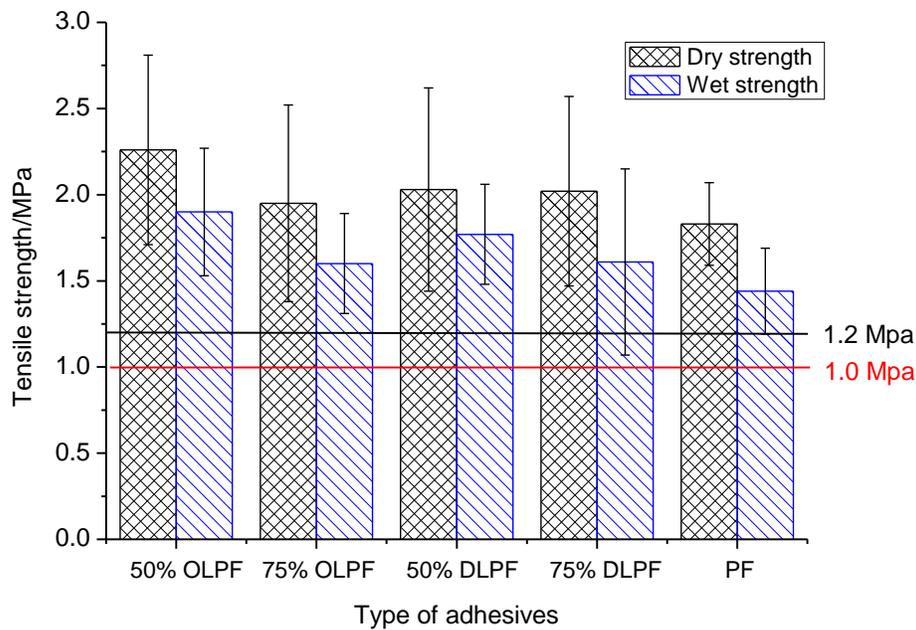
**Figure 7-5.** Tensile-strength profile of plywood glued by OLPF, DLPF and PF adhesives.
