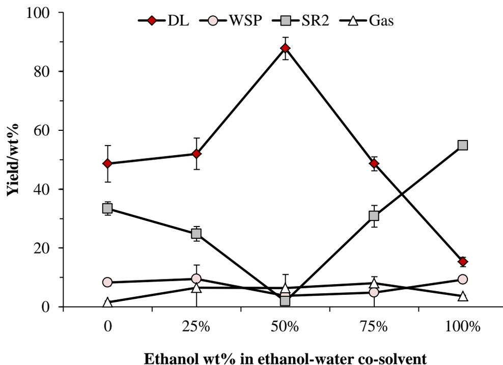
**Figure 6-1.** Effects of ethanol concentration on the yields of DL, WSP, SR<sub>2</sub> and Gas obtained at 300 °C for 4 hr in a 14 mL micro reactor.
