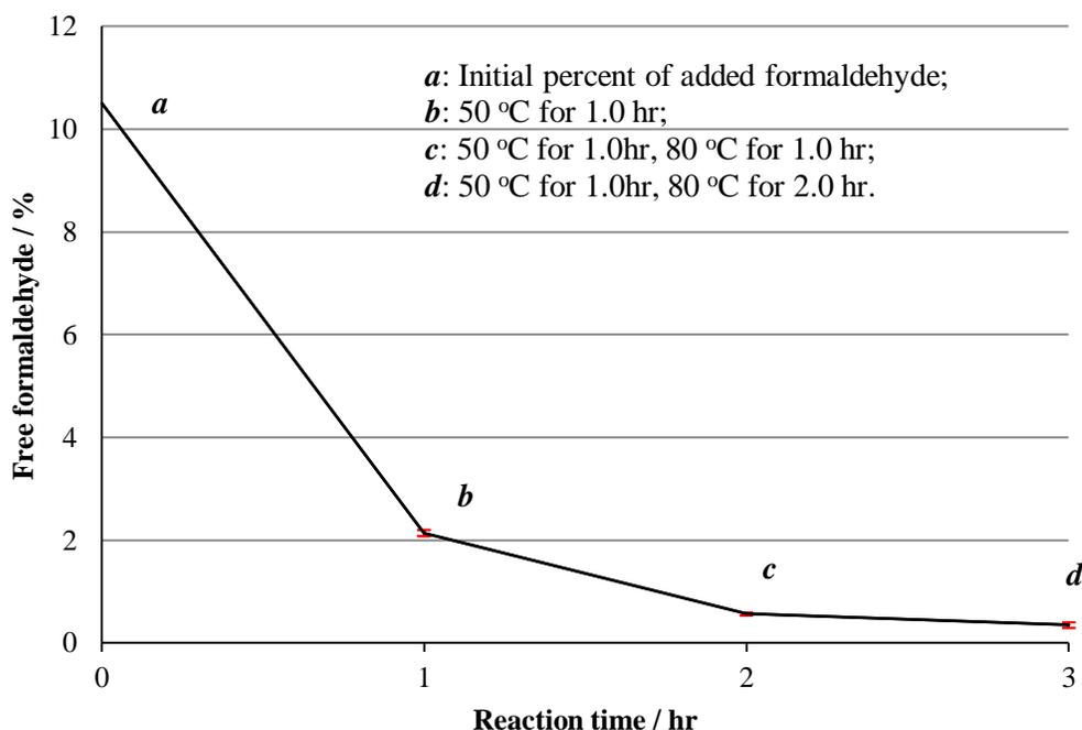
**Figure 5-3.** Free formaldehyde levels during the process of methylation treatment.
