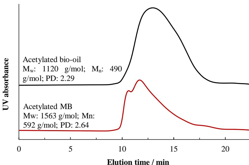
**Figure 5-2.** GPC spectra of the raw bio-oil and the MB after acetylation (PD =  $M_w/M_n$ : Polydispersity).
