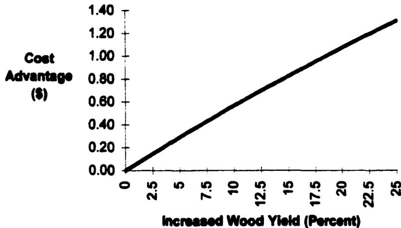
Figure 26. Relationship between increasing the yield of the FT-SW harvesting system and the marginal cost advantage of reduced hauling costs for the Wabigoon and English River forests.
