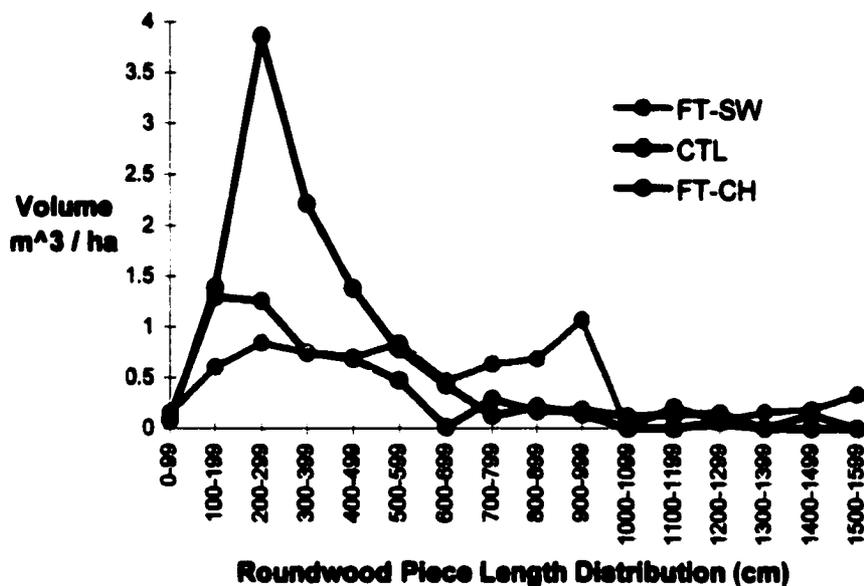
Figure 22. Volume of cutover roundwood pieces distributed by 100 cm length class for the FT-SW, CTL and FT-CH systems.
