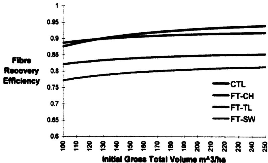
Figure 25. Expected fibre recovery efficiency across a range of initial gross total volumes of four common harvesting systems; FT-SW, (feller-buncher/skidder/delimiter/slasher), FT-CH (feller-buncher/skidder/delimiter-debarker-chipper, CTL (single-grip harvester/forwarder), and FT-TL (feller-buncher/skidder/delimiter).
