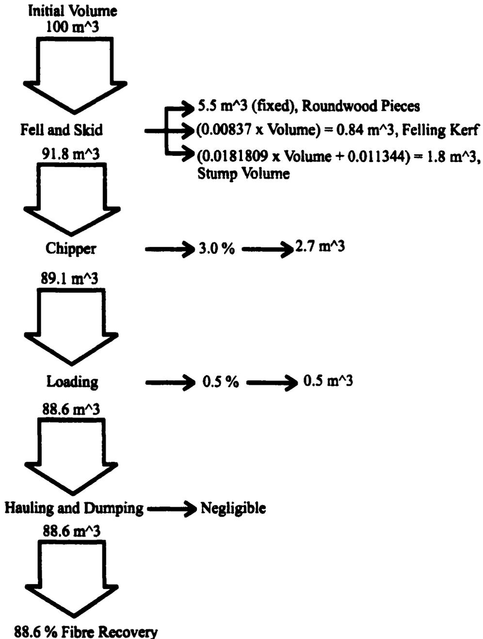
**Figure 14. Wood fibre utilization model for the FT-CH system (feller-buncher/skidder/delimiter-debarker-chipper). Descending arrows are to scale and indicate wood flow towards the mill. Horizontal arrows indicate fibre losses. The initial volume of 100 m<sup>3</sup>/ha is used as an arbitrary seed value.**
