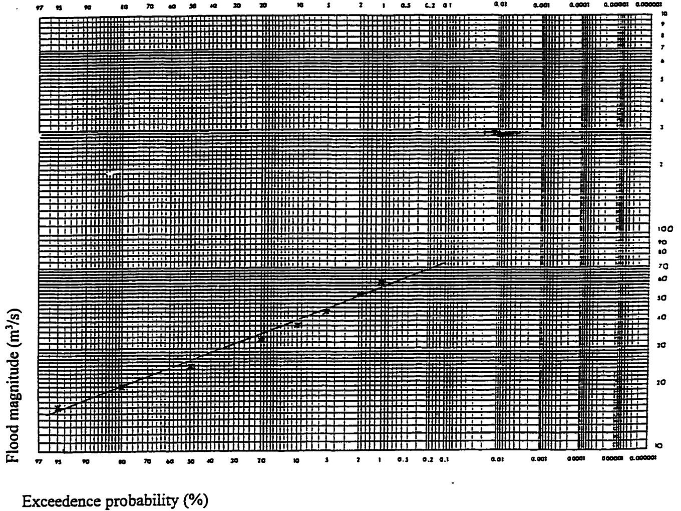
Figure 15. Flood frequency regime obtained by GEV distribution for Garu station
