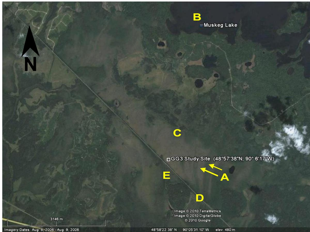
Figure 1.2: The GG3 peatland showing patterning typical of water track fens (A). Water flows from the height of land at Muskeg Lake (477 m B) south, through headwater wetlands (C) to the GG3 study site (labeled). Road access (D) and main drainage point (471 m E) are indicated.
