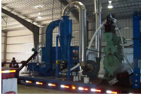
Figure 1.4: Proprietary mechanical dewatering equipment used by Peat Resources Ltd. to pelletize wet peat is transportable to a site via a flat bed truck.
