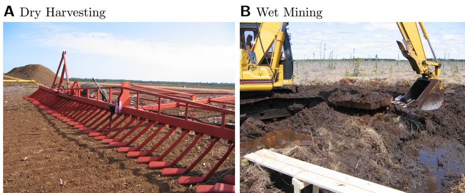
Figure 1.3: Contrasting techniques used to extract peat. **A** Dry harvesting as observed during a peatland restoration tour in northern Minnesota (2008). The “hockeys” (see text) are exposing a new peat layer for drying (foreground), while harvested peat is stored in piles (background). **B** Wet mining as employed during this research (2008). A backhoe sits atop a floating mat and extracts higher energy, catotelm peat.
