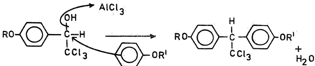
Scheme 1. Reaction mechanism for the formation of the diaryltrichloroethanes.
