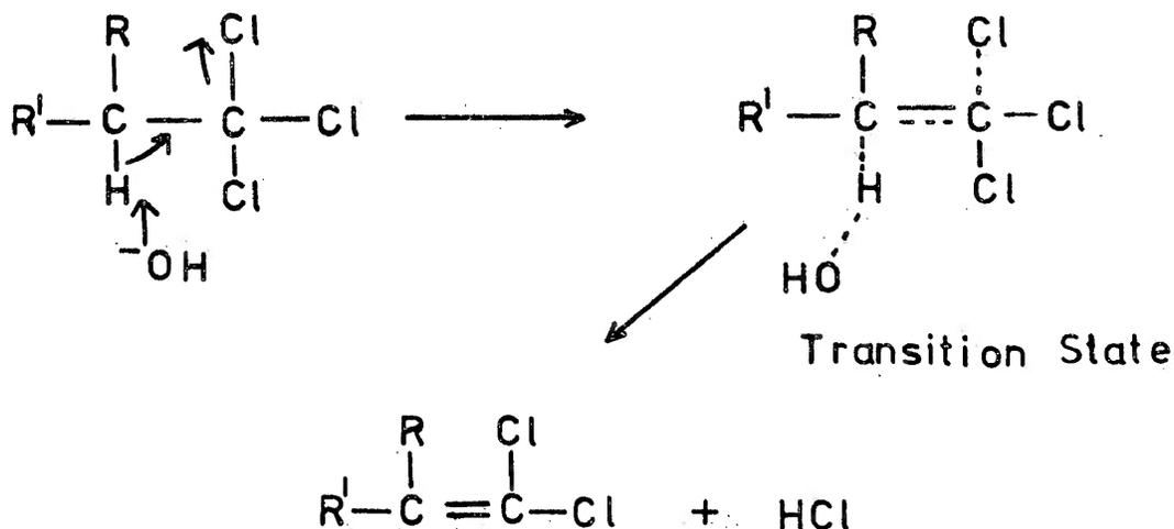
Scheme 3. Reaction mechanism for the formation of the diaryldichloroethylenes.
