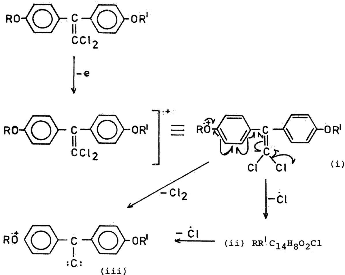
(i)  $\text{R} = \text{R}' = \text{CH}_3$ :  $m/e$  308;  $\text{R} = \text{CH}_3$ ;  $\text{R}' = \text{H}$ :  $m/e$  294;
