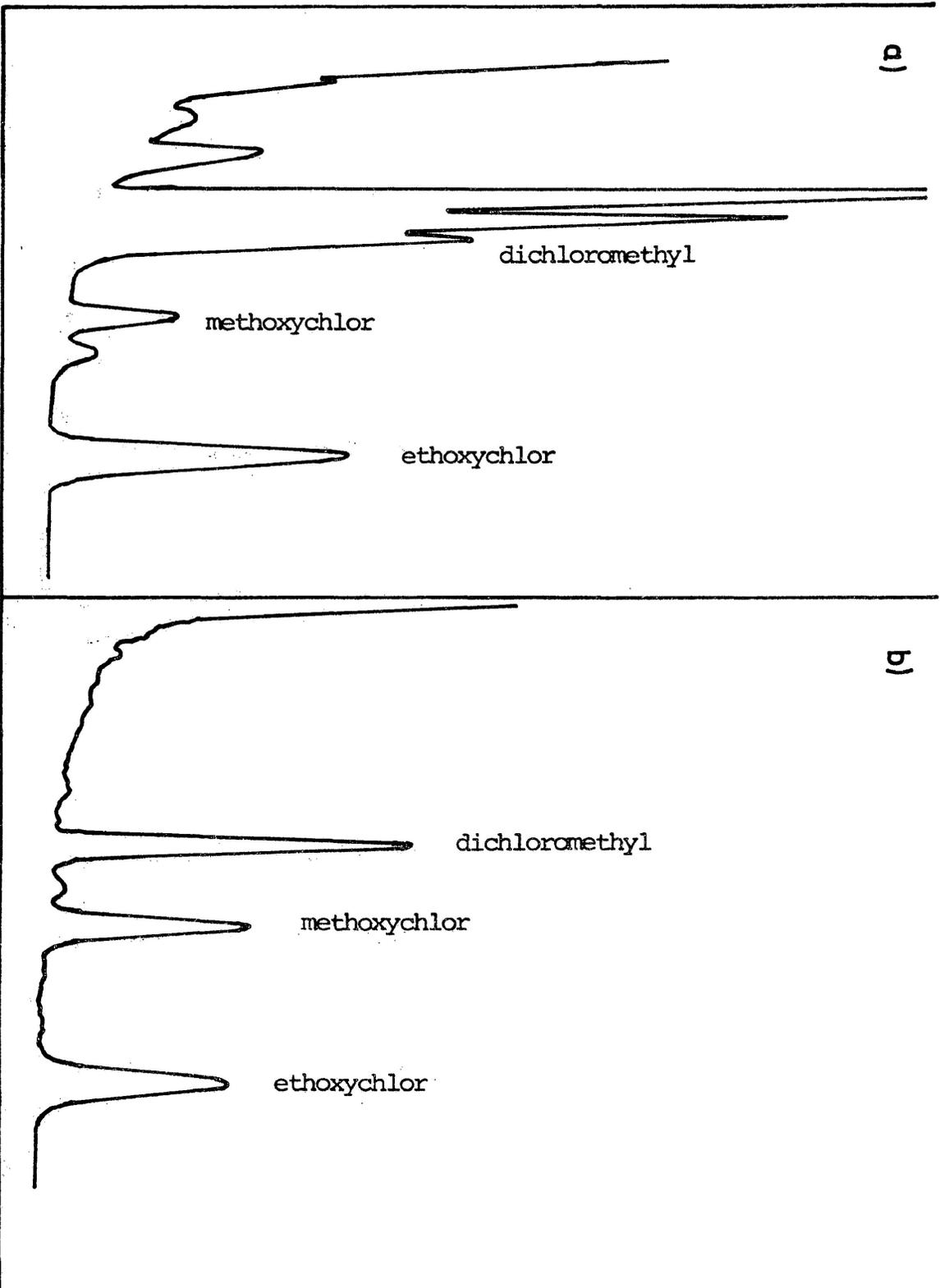
FIG. 9 Result of cleanup process for extracts of *K. pneumoniae* incubated with methoxychlor on the SE-30(5%) column. a) before cleanup; b) after cleanup.
