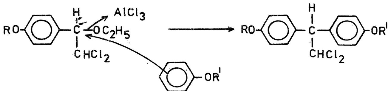
Scheme 4. Reaction mechanism for the formation of the diaryldichloroethanes.
