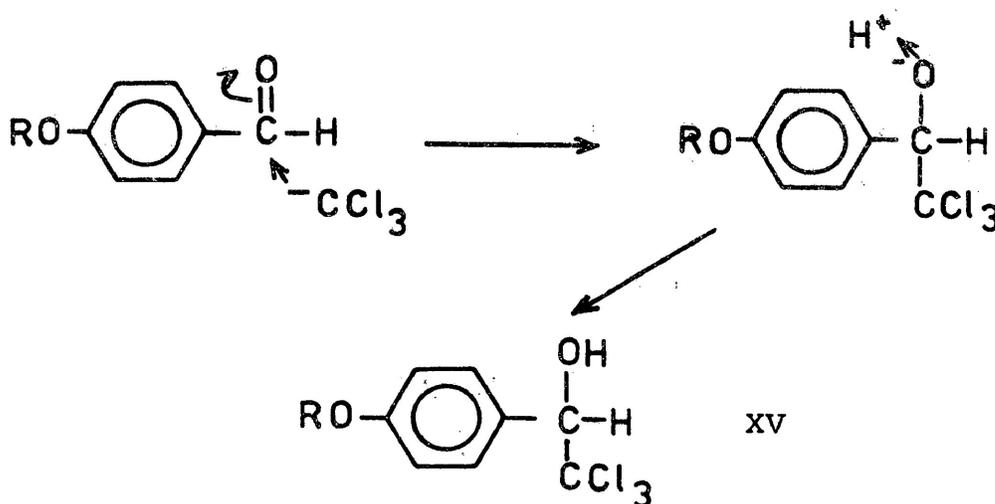
Scheme 2. Reaction mechanism for the formation of the *p*-methoxyphenyl-1,1,1-trichloroethanol, (XV).
