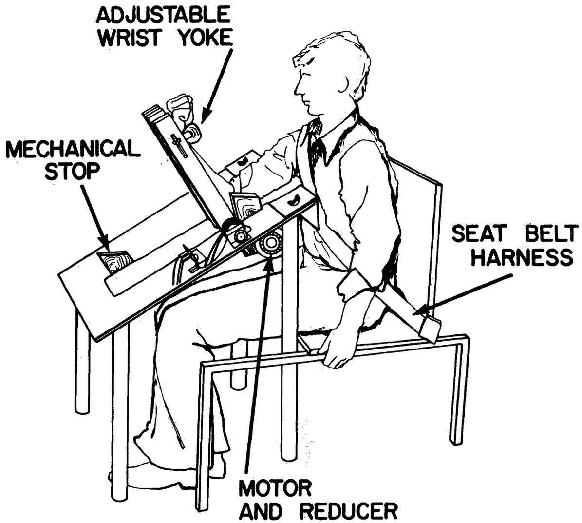
Figure 1. Dynamometer for Testing and Training.
