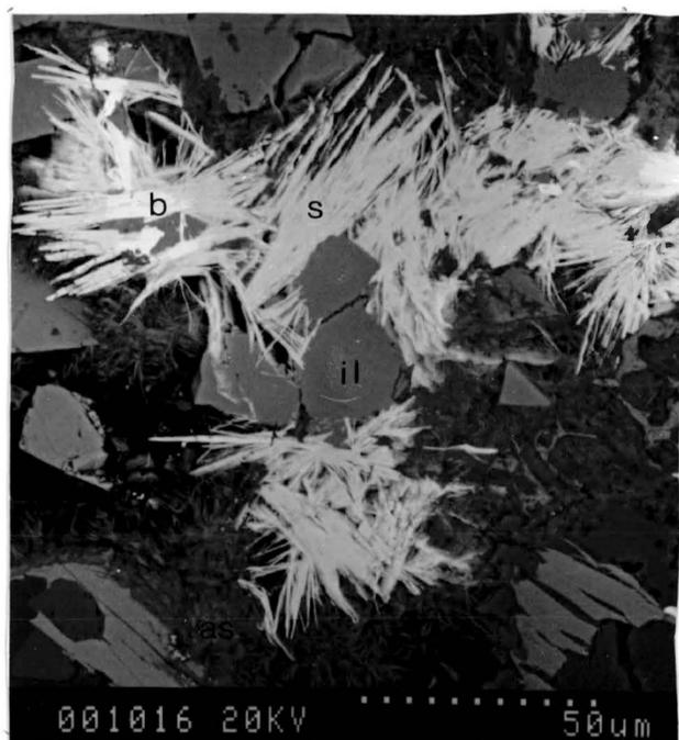
Fig 2.9 and 2.10. [ Centre III, ferro-edenite syenite, Neys - Ashburton Lookout area]. Acicular synchysite (s) surrounding ilmenite (il) replaces alteration silicate (as). Synchysite rarely nucleates on bastnaesite (b) (sample # C2122).
