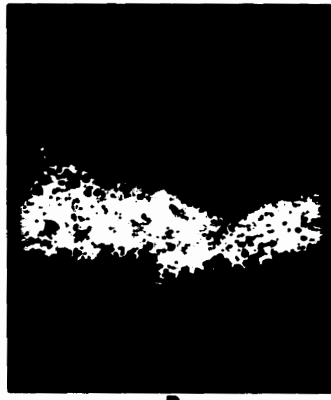
Figure 3.09 SEM photomicrographs taken from core present in the Keewatin Hematite Lakes area. A) Chert-interbedded with carbonate. B) Chert-magnetite iron formation (chert-black, magnetite-white). C) Chert-magnetite iron formation. D) Sulphide-chert iron formation (chert-black, sulphide-white).
