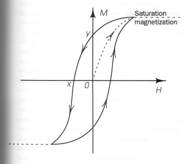
Figure 3.01. Hysteresis loop of a ferromagnetic material. The remanence is indicated by y. The coercive force is indicated by x (from Mulay, 1963).
