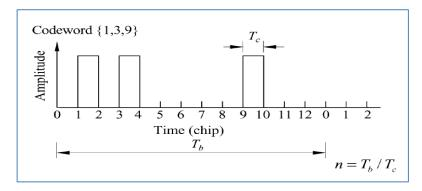
Figure 2.11: Codeword. Illustration courtesy of [7].
