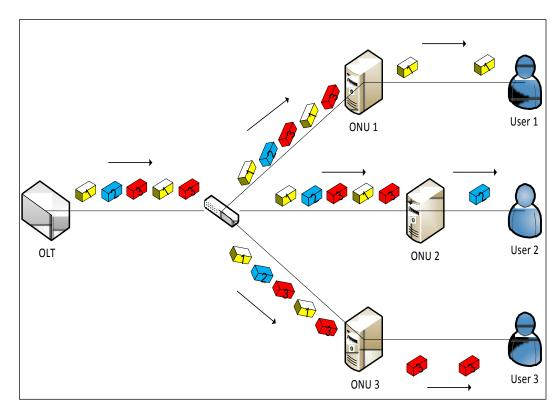
Figure 2.2: Downlink Direction of PON. Illustration courtesy of [11].
