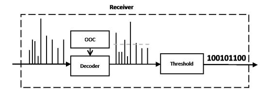
Figure 2.8: Incoming Data Stream at the Receiver
