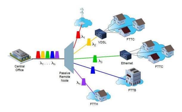
Figure 2.4: WDMA-PON where each end-point is assigned a dedicated wavelength for communication. Illustration courtesy of [18].
