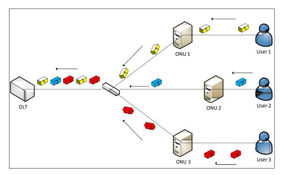
Figure 2.3: Uplink Direction of PON. Illustration courtesy of [11].
