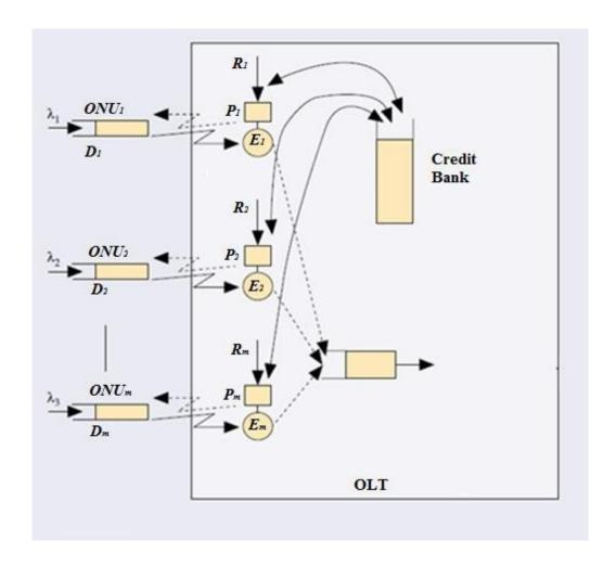
Figure 3.2: The Leaky Bucket structure for uplink traffic.
