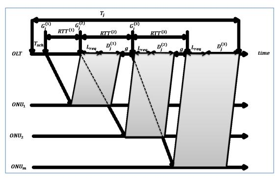
Figure 3.4: Illustrative Example of a Transmission Cycle [34]
