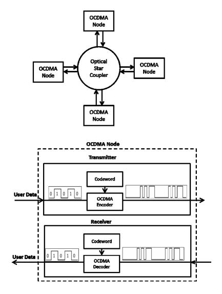
Figure 2.5: Code-Division Multiple-Access Optical System.
