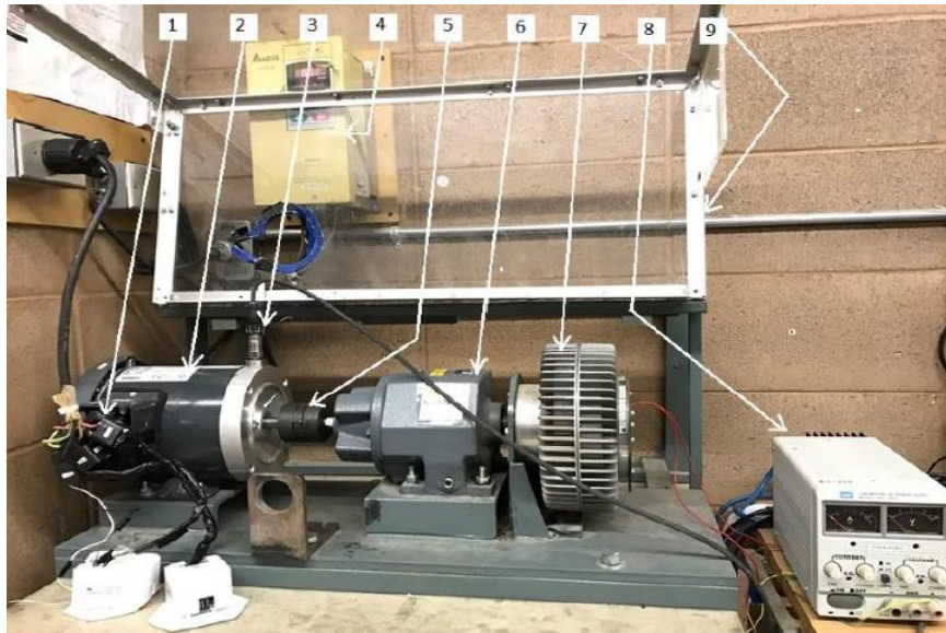
Fig. 3.4 Experimental setup [2]: (1) Smart current sensors; (2) IM; (3) Vibration sensor; (4) Power supply with VFD; (5) Elastic coupling; (6) Gearbox; (7) Dynamometer; (8) DC supply for dynamometer; and (9) Enclosure.
