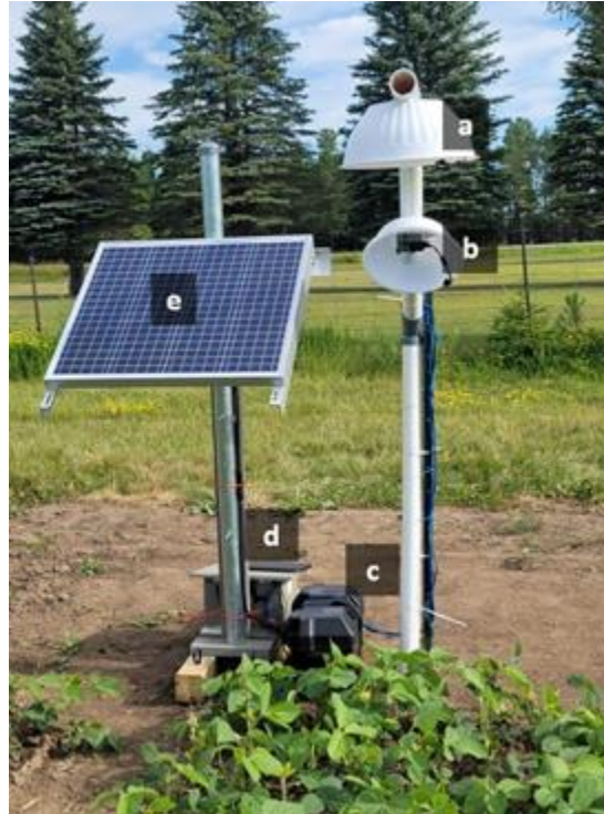
Figure 2.2: The camera setup: (a) the camera oriented at 90°; (b) the camera oriented at 45°; (c) the power supply (battery and the box); (d) the wooden box for the Raspberry Pi computer, controller and other accessories; and (e) solar panel.
