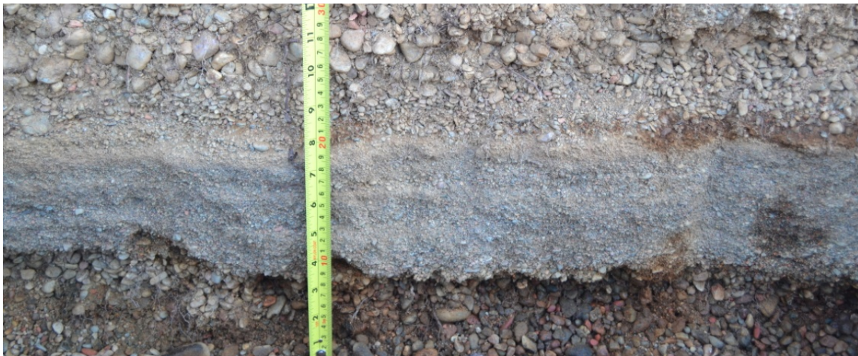
Figure 5.104. Lithofacies 3 underlain by massive open framework pebbles, overlain by a thin silt layer (lithofacies 1) and lithofacies 3 at the top.
