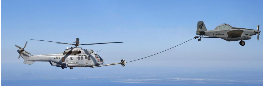
Figure 2.1: Concept of plane-to-helicopter aerial refueling with a probe-drogue system [77].
