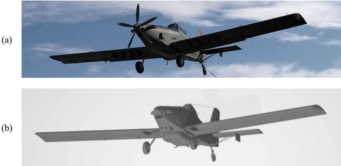
Figure 2.9: Aircraft modeling: (a) reference AT-802F [95]. (b) 3D model of FuelBoss with auxiliary fuel tank.
