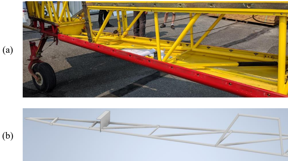
Figure 2.10: Fuselage modeling: (a) FuelBoss rear fuselage, (b) 3D model of the FuelBoss rear fuselage internal structure.
