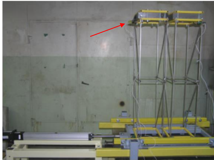
Figure 2.15. Overview of the experimental setup of the shaking table and adjacent framed structures with different top-mounted properties, adopted from (Jankowski, 2010)
