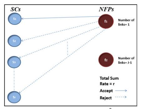
Figure 3.3: SCs ask NFPs to associate using  $(DM)^2S$  algorithm
