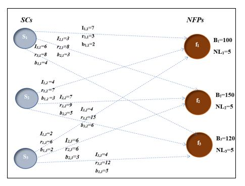
Figure 4.2: Example of the interference, data rate and bandwidth between SCs and NFPs.
