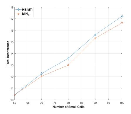
Figure 4.7: Total interference with  $SC_{rm_j} = (30-60)$  Mbps and  $NL_i = J/5$ .
