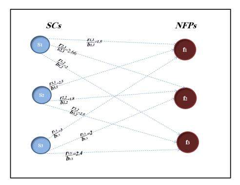
Figure 4.3: The ratio between data rate and the bandwidth
