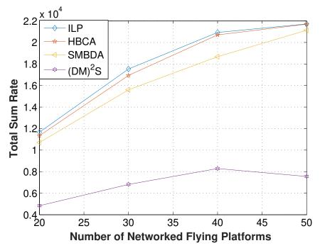
Figure 3.18: Total Sum Rate versus the number of NFPs for the proposed HBCA, SMBDA, ILP, and  $(DM)^2S$  at 100 SCs.
