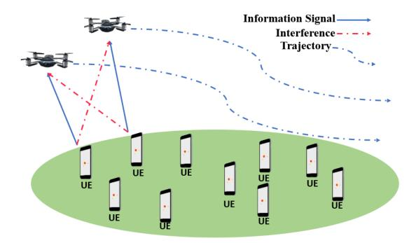
Figure 5.1: A multi-UAVs enabled wireless network.
