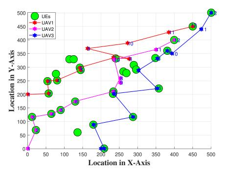
Figure 5.4: The trajectory of 3 UAVs flying over 30 UEs for offline scenario.
