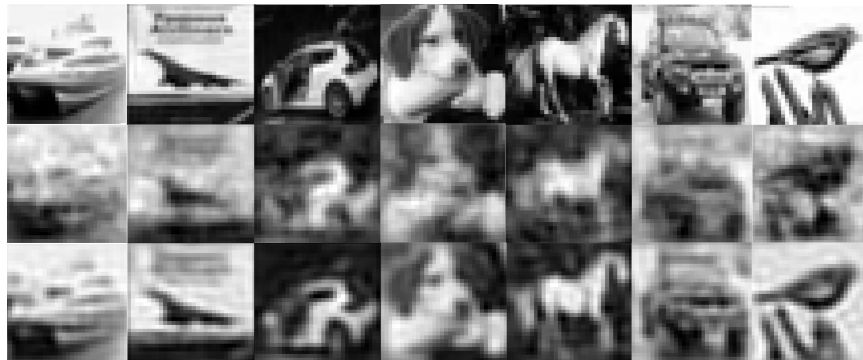
Figure 4.9: The qualitative comparisons of small image reconstruction performance of deep autoencoder and our proposed algorithm. From top to bottom: some images randomly sampled from CIFAR10 testing set; the corresponding deep autoencoder reconstructed images; the corresponding OS-Autoencoder reconstructed images.
