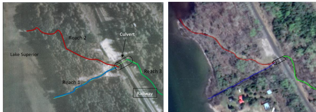
Source: Left, Kaurin (2015). Right, Google maps Figure 1: Kama Creek reach locations. Blue, reach 1 is post 1962 channelization and pre 2011 remediation. Red, reach 2 is pre 1962 channelization (historic condition) and post 2011 remediation. Green, reach 3 is the stream above the culvert crossing.
