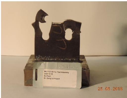
T127-45-1-a: bearing tear-out
