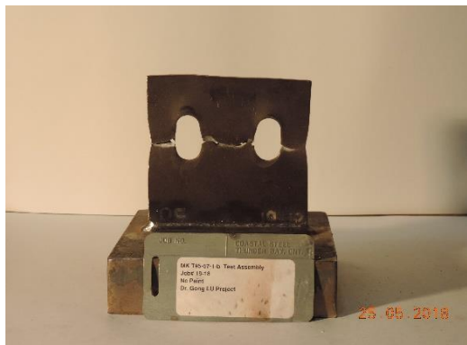
T95-57-1-b: net-section rupture
