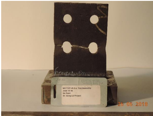
T127-45-2-a: net-section rupture
