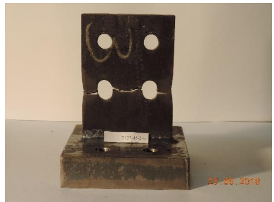
T127-45-2-b: net-section rupture
