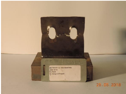
T95-57-1-a: net-section rupture
