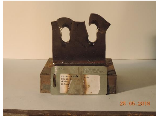
T95-45-1-b: bearing tear-out
