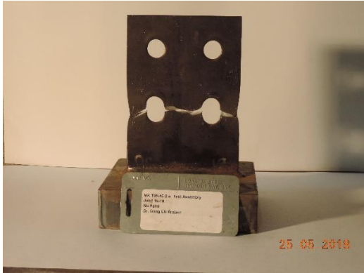
T95-45-2-a: net-section rupture
