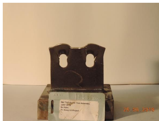
T127-45-1-b: bearing tear-out
