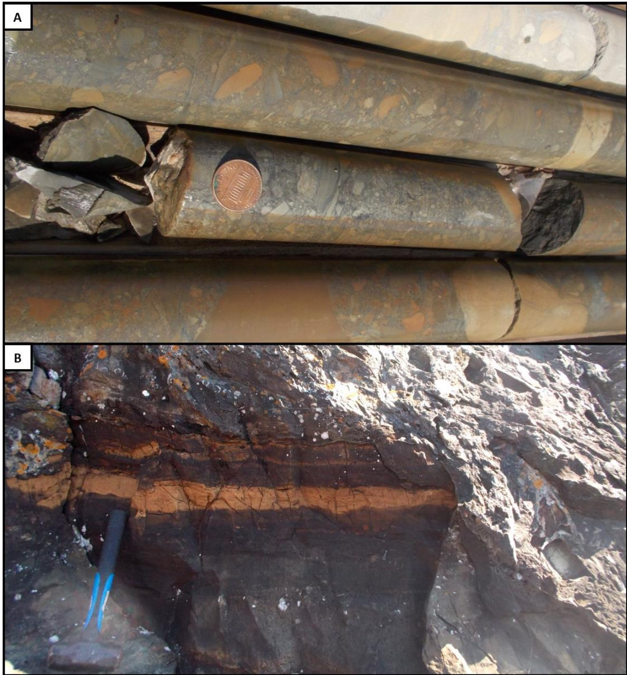
Figure 63: A: Intrusive breccia in drill hole 105-2. Clast size is highly variable, ranging from 1mm up to several cm, and clasts are randomly oriented throughout. B: Outcrop of the Interbedded ferruginous carbonate and siltstone lithofacies association that has become intruded by a breccia.
