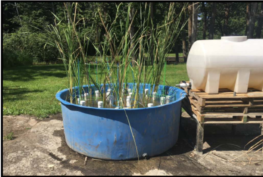
Figure 11. Mesocosm set up with cattail planted (n=6) and unplanted (n=6) treatments with reservoir tank
