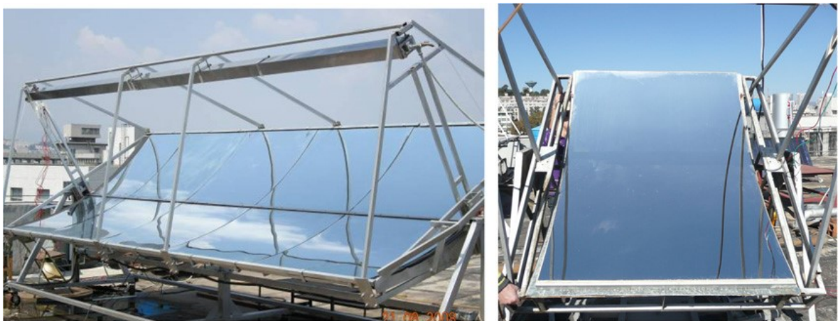
Figure 2.2: The 10 m 2 Trough Concentrating PVT (TCPVT) with Supercell, GaAs and Si cell array at receiver and high reflectivity concentrating mirrors of reflectivity 0.69 and 0.92 analyzed by M. Li et al. [46].
