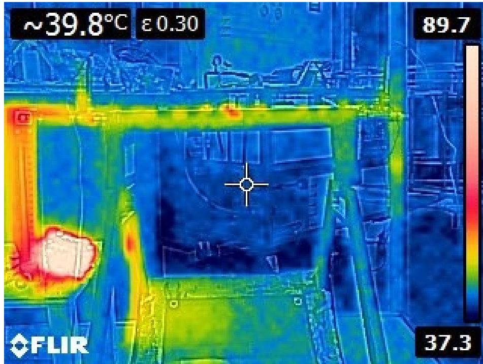
Figure 4.4: Thermal image of the thermal collector when only air blower is circulating the air.
