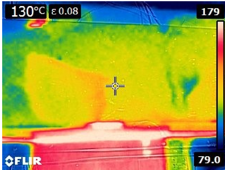
Figure 4.10 a: Infrared image of the top black surface captured with FLIR IR camera calibrated for the surface emissivity for indoor testing.
