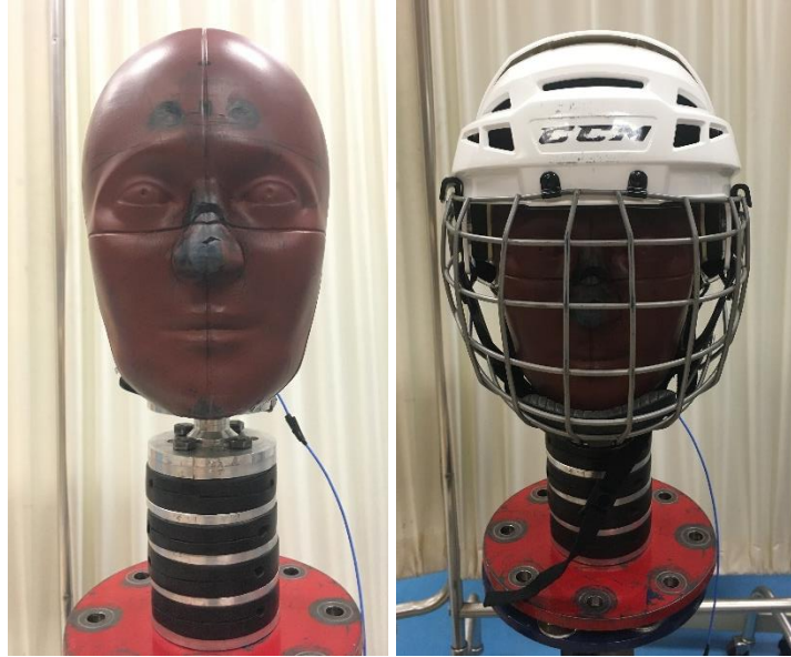
Figure 8. The NOCSAE headform. The headform is designed to represent the 50 th percentile of an adult head and has anatomically correct bone structure and facial features. The headform was equipped with a medium-size CCM VO8 helmet.
