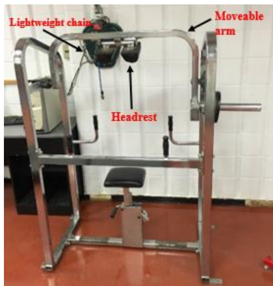
Figure 5. The Nautilus neck strength machine. The lightweight chain attached the load cell to the headrest and prevented the moveable arm from moving during the isometric contractions.
