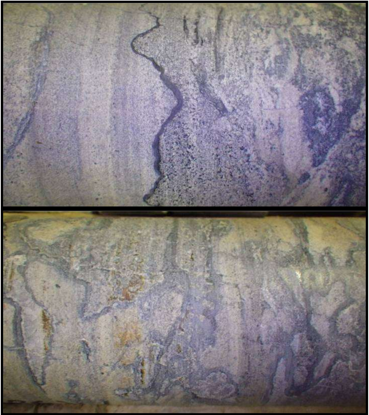
Figure 201. (Upper) Fine-grained carbonate grainstone with pronounced stylolites. Figure 202. (Lower) Very fine-grained grainstone and silt layers that are very diagenetically altered.
