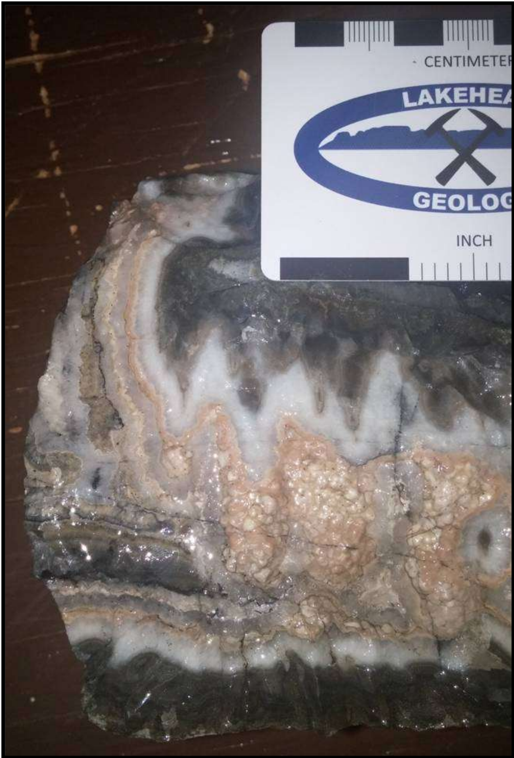
Figure 176. Side view of silica stalactite sample extracted from Terry Fox. Stalactites hang from 'ceiling' and develop a botryoidal coating on each stalactite finger.
