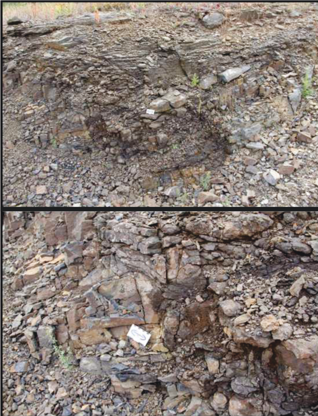
Figure 43. (Above) Photo of ditch outcrop in Harbour Expressway. Figure 44. (Below) Lenticular-bedded shaley layers in Harbour Expressway.
