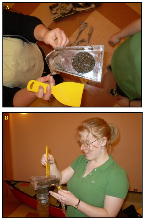
Figure 5.6 Sampling the short core, WTFSH08-02, to be sub-sampled later for pollen and phytoliths processing in the lab.
