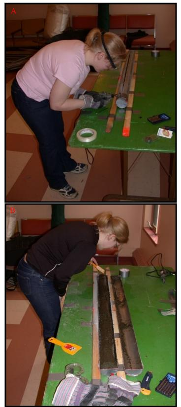
Figure 5.4 Photo A) Splitting the core barrel, photo B) examining the sediments.
