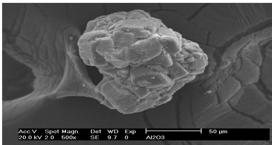
Fig 3.2. SEM micrograph of unloaded \gamma -Al 2 O 3 calcined at 600 °C
