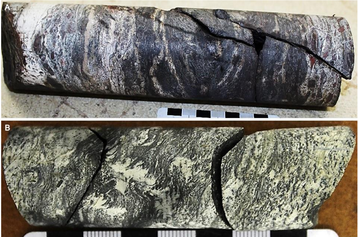
Figure 73. Photographs of stromatolites in the 2627 core. (A) At the base of the stromatolitic horizon, undulatory laminae 2-4 mm thick make up a 15 cm thick stratiform mat. The mat overlies coarse-grainstone containing abundant jasper rip-up clasts in a white chert cement (up direction to left). (B) Cream and dark green chert make up the stromatolites in the upper 100 cm stromatolitic horizon.
