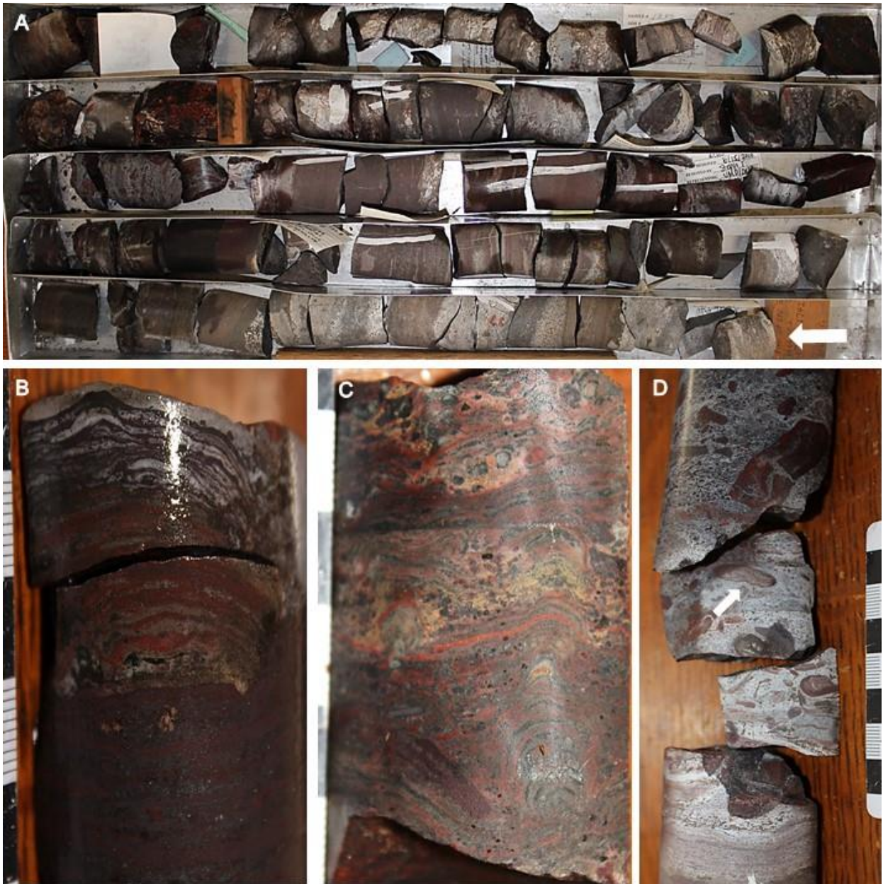
Figure 72. Photograph of MGS-2 Core. The Upper Stromatolitic Unit is 110 cm thick, and consists of three distinct stromatolitic horizons separated by decimeter scale layers of chemical mud intercalated with medium-grainstone; white arrow indicates up direction, (a) is at the top of the section. (B) The basal stromatolites consist of columnar, stratiform and pseudocolumnar forms composed primarily of millimeter-scale jasper laminae alternating with cream to white chert. (C) The middle stromatolite contains well developed digitate forms overlain by stratiform mats containing abundant trapped grains within the laminae. (D) The top horizon contains chert rip-up clasts with rare centimeter-scale oncolites (white arrow).
