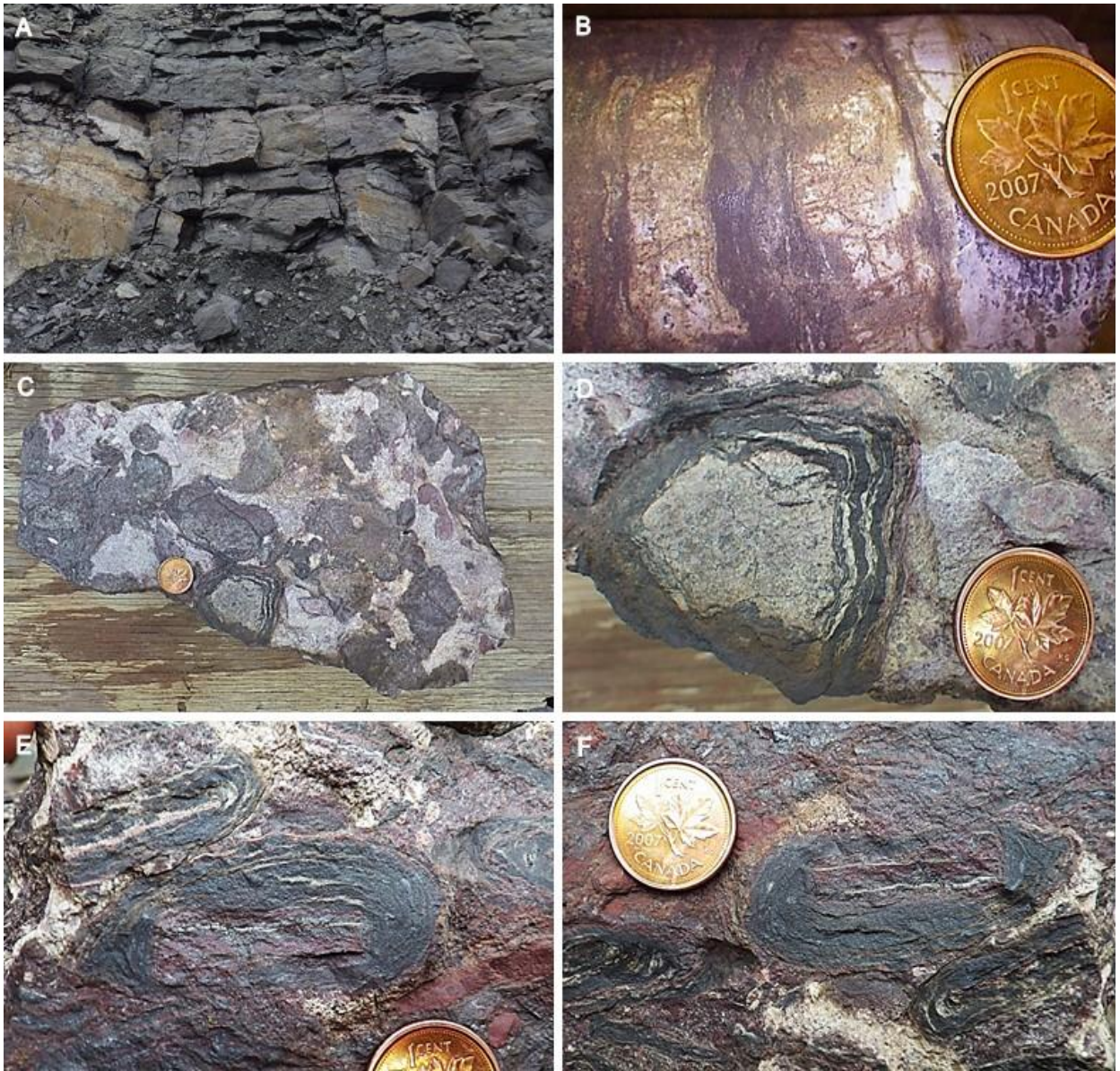
Figure 58. Photographs of the UTAC Thunder Bird North oncolites. (A) The UC-6 oncolite subunit ranges in thickness from 70-100 cm and is continuous throughout the mine. (B) In core the oncolites appear as wavy dark layers which alternate with white chert. (C) The oncolites are surrounded by a mottled, coarse-grained grainstone. (D) The oncolites occur as subrounded spheres, 4 to 8 cm in diameter and made up of millimeter-scale light granule-rich and dark iron-rich layers. (E-F) More commonly the oncolites occur as centimeter-scale elongated spheres composed of an angular chert grain surrounded by dark laminae.
