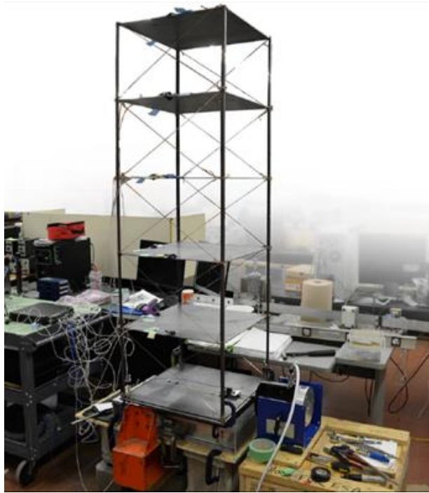
Figure 4.17: Braced structure resting on top of the shaker table.
